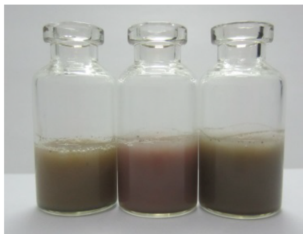
Fig. S1. The pictures of IO@PLA/GO dissolved in serum (left), culture medium (middle) and water (right).
