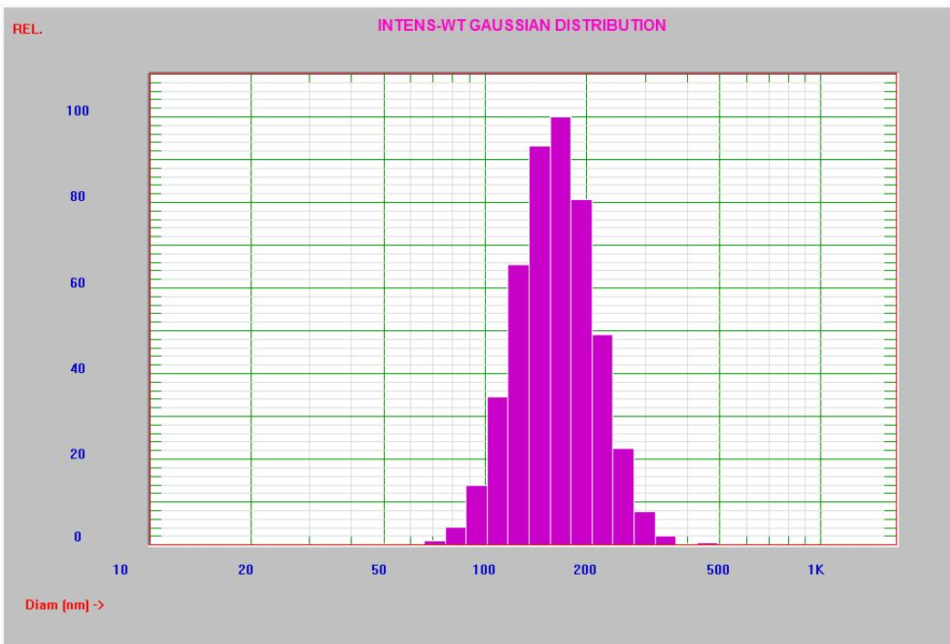
**Fig. S9** DLS measurement: PPE-NP-10 nanoparticles.
