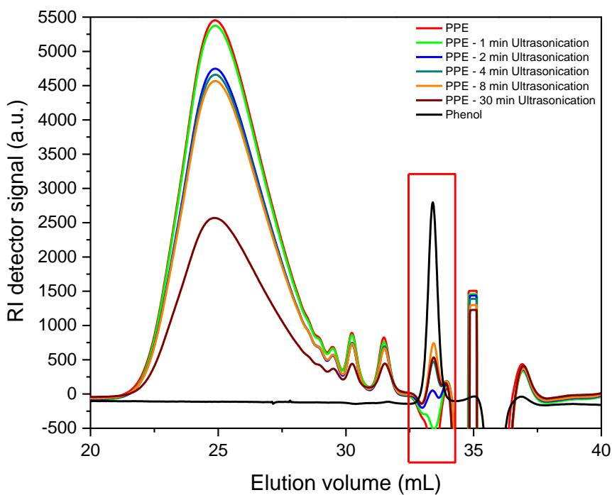
**Fig. S24** RI detector signal from the GPC elugram for the polymer PPE after the application of ultrasound (1/4" tip; 70% amplitude; 30 s on and 10 s off) for different periods of time and for phenol.
