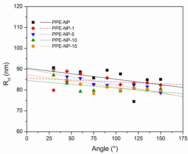
**Fig. S2** Multi-angle DLS scattering of the “placebo” PPE nanoparticles and the Paclitaxel loaded PPE nanoparticles formulations.
