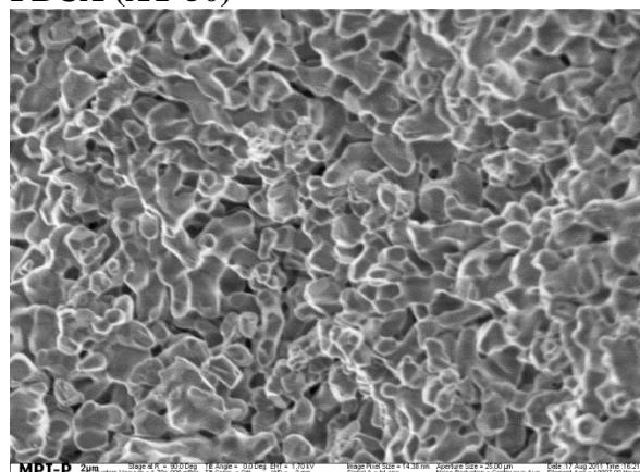
**Fig. S23** SEM images of biphasic calcium phosphate granules, MBCP+ (80-200 µm) probed with different nanoparticles.
