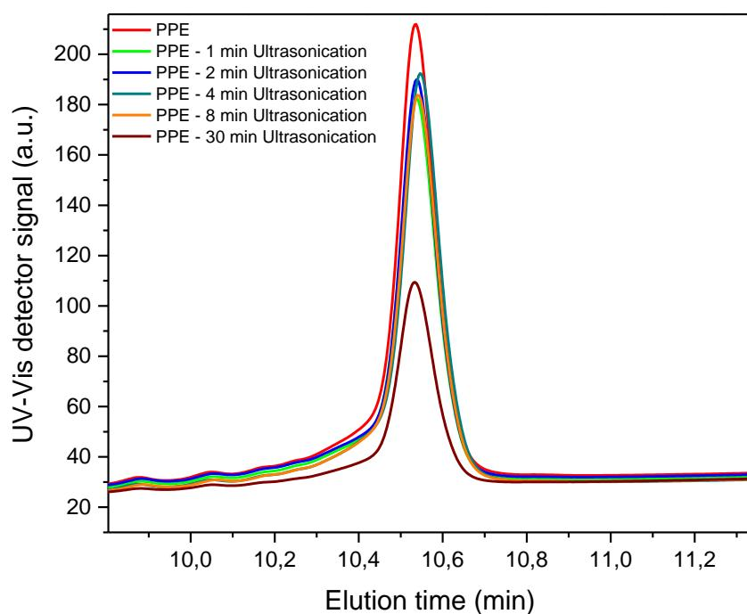
**Fig. S25** UV-Vis detector signal from HPLC elugram for the polymer PPE after the application of ultrasound (1/4" tip; 70% amplitude; 30 s on and 10 s off) for different periods of time.
