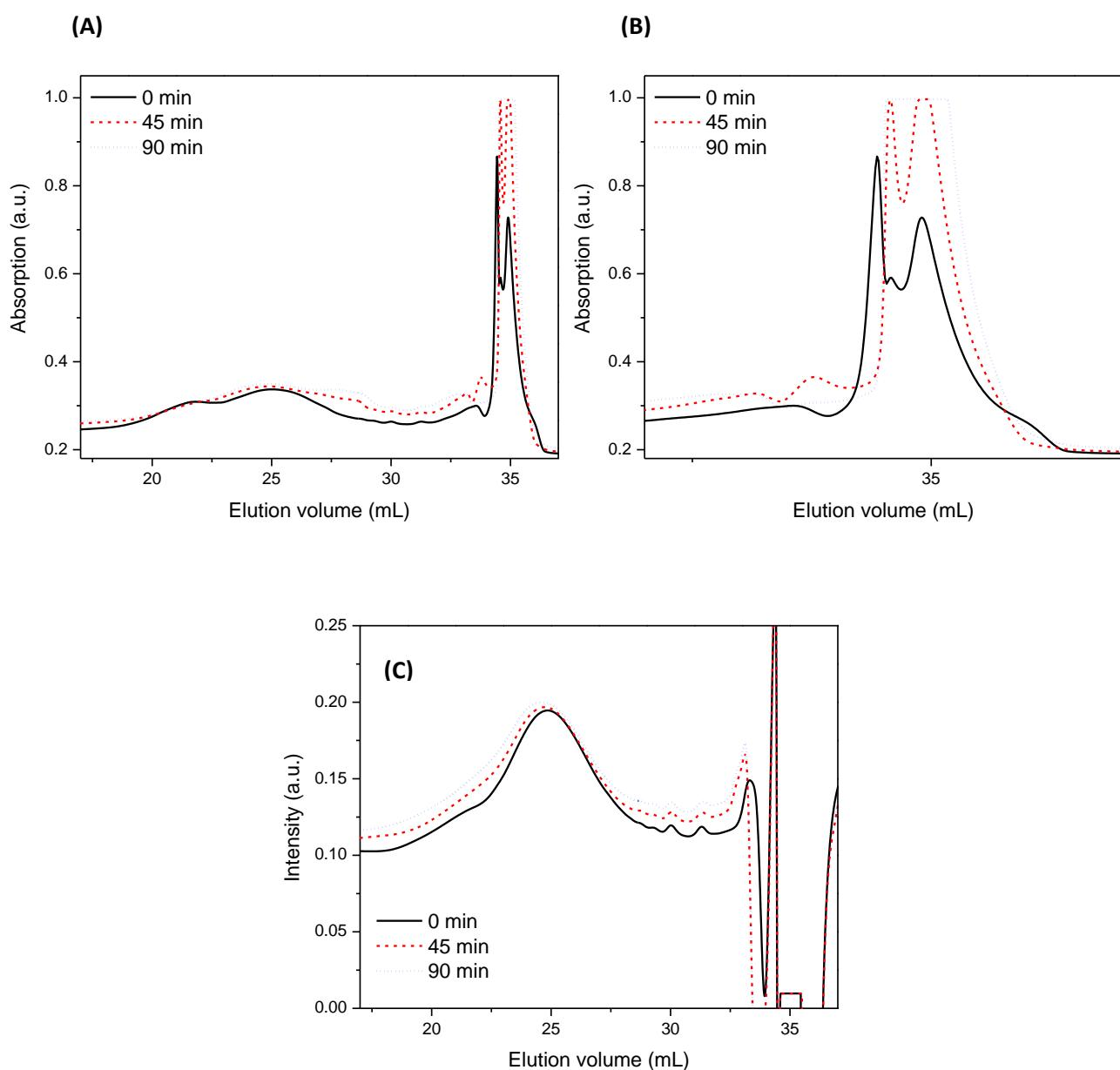
**Fig. S18** GPC elugrams for the polymer PPE in THF and 0,1 M HCl: (a) and (b) UV-Vis signal; (c) Refractive Index signal.
