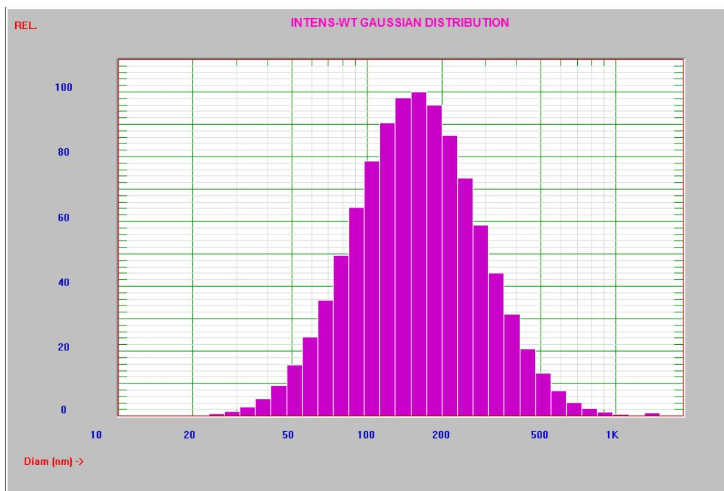
**Fig. S10** DLS measurement: PPE-NP-15 nanoparticles.
