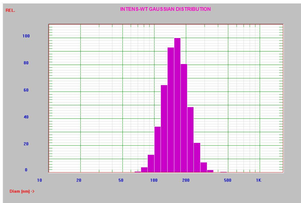
**Fig. S7** DLS measurement: PPE-NP-1 nanoparticles.
