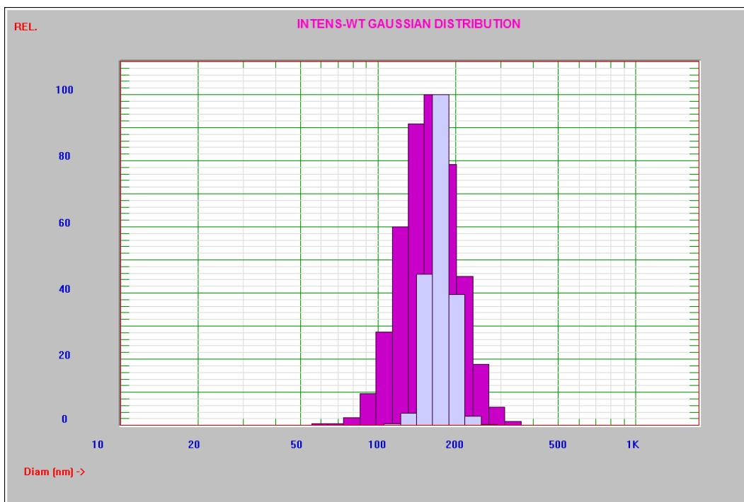
**Fig. S3** DLS measurements of a first batch PPE-NP nanoparticles: before (blue) and after (pink) 2 months kept at 4°C and pH 7.
