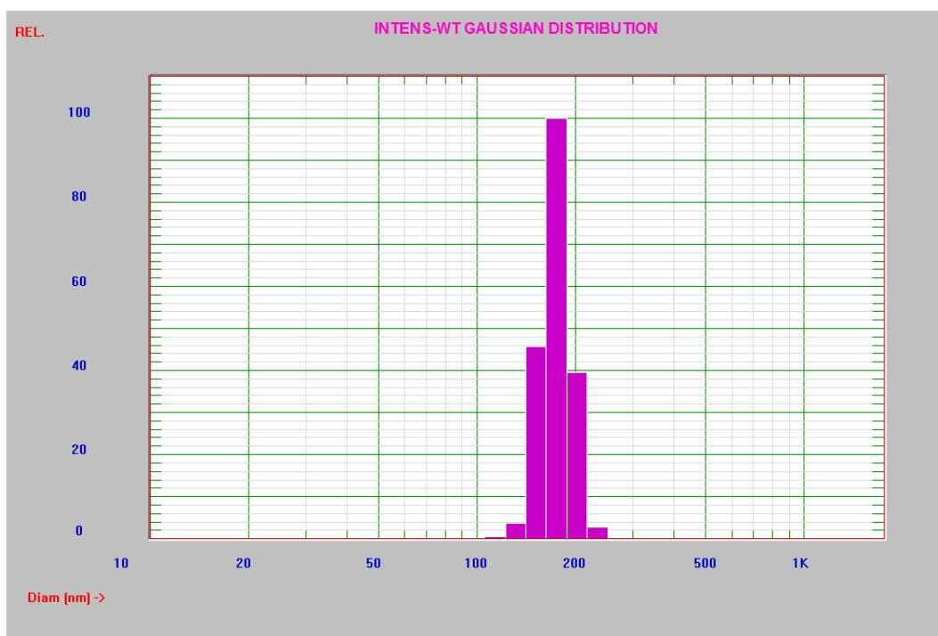
**Fig. S6** DLS measurement: PPE-NP nanoparticles.
