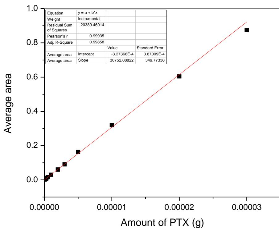
**Fig. S20** HPLC calibration curve constructed from Paclitaxel in THF:0,1 % aqueous TFA (80:20) stock solutions.
