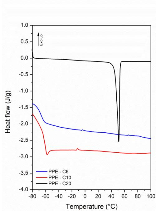
**Fig. S1** DSC curves for of the saturated polyphosphoesters PPE-C6, PPE-C10 and PPE-C20.
