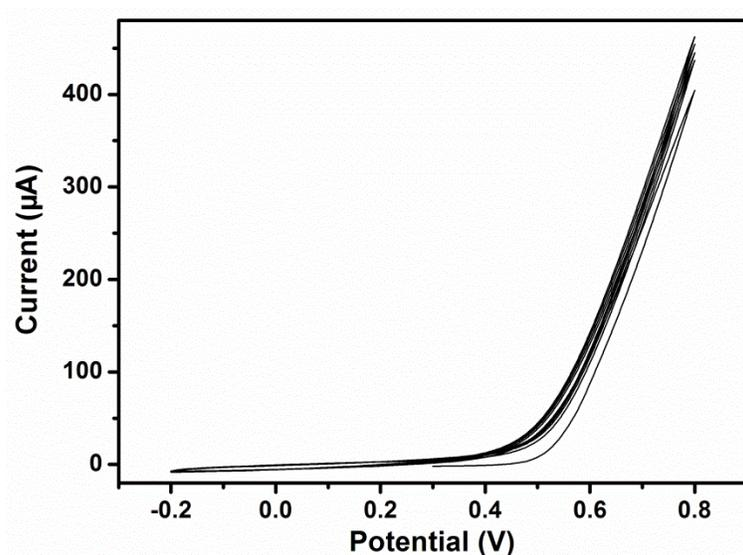
**Figure S1.** Cyclic voltammograms recorded during the pyrrole electropolymerization on the CHI/VSG scaffold.
