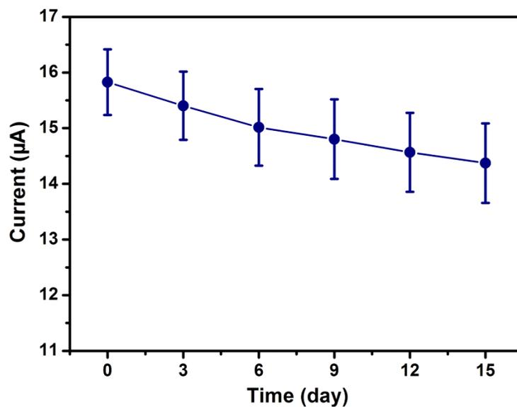
**Figure S5.** The DPV current response of the CHI/VSG/PPy sensor in 0.1 M PBS containing 40 µM DA for 15 days.
