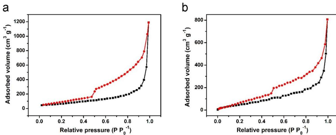
**Figure S3.** N<sub>2</sub> adsorption-desorption isotherm of the CHI/VSG and CHI/VSG/PPy.
