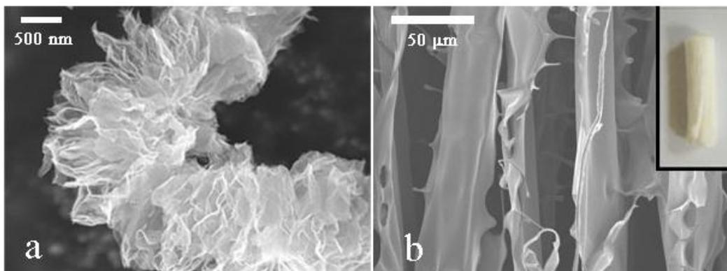
**Figure S2.** FESEM image of pure VSG powder (a) and CHI scaffold (b), inset of (b) is the photograph of CHI scaffold.
