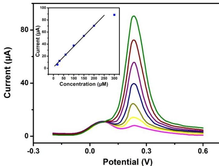
**Figure S4.** DPVs of DA at the CHI/VSG/PPy electrode in the presence of 0.2 mM AA in 0.1 M PBS (pH=6.0). From bottom to top DA concentration= 20, 30, 60, 100, 150, 200, 300 µM. Inset: the relation between the peak current and the DA concentration.
