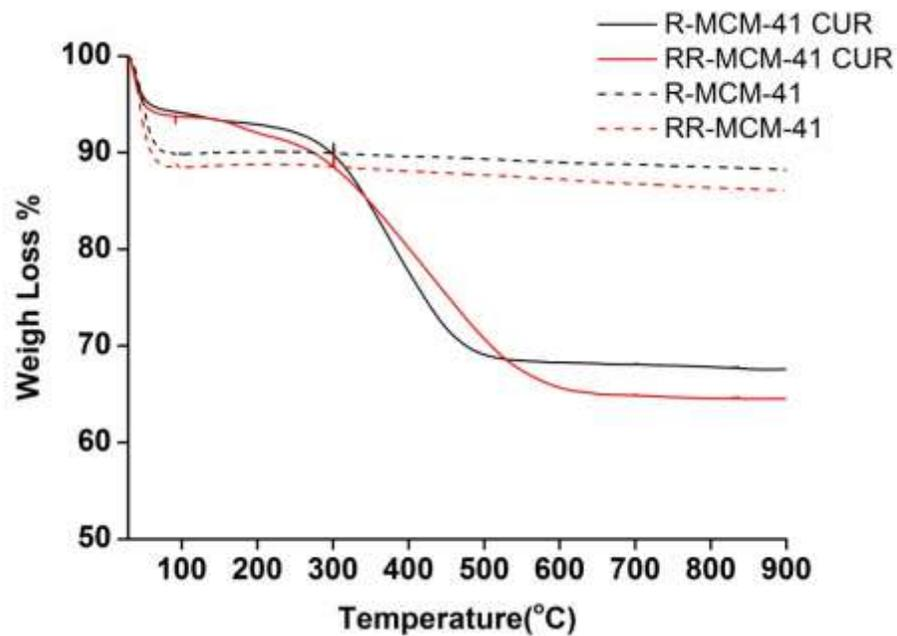
**Figure S3.** Thermogravimetric analysis of R-MCM-41 CUR, RR-MCM-41 CUR, R-MCM-41 and RR-MCM-41.
