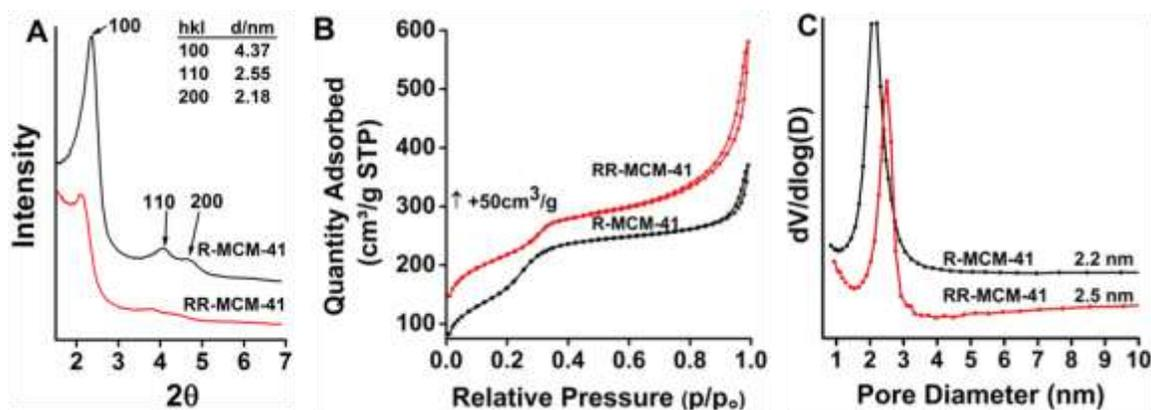
Figure S1. Small-angle XRD patterns (A), nitrogen adsorption-desorption isotherms (B) and pore size distribution plot of R-MCM-41 and RR-MCM-41.
