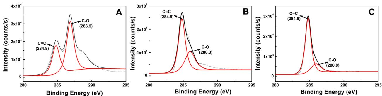
**Fig. S3.** High-resolution XPS of C 1s spectra of (A) GO, (B) TB-rGO and (C) Fc-rGO.
