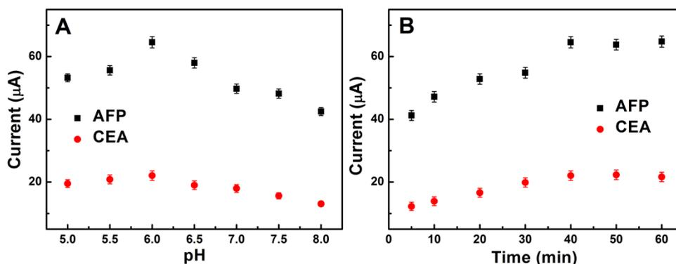
**Fig. S5.** Effect of pH of detection solution (incubation time 1 h) (A) and incubation time (detection solution pH=6.0) (B) on SWV responses to  $1 \text{ ng mL}^{-1}$  CEA and AFP at the immunosensor array.
