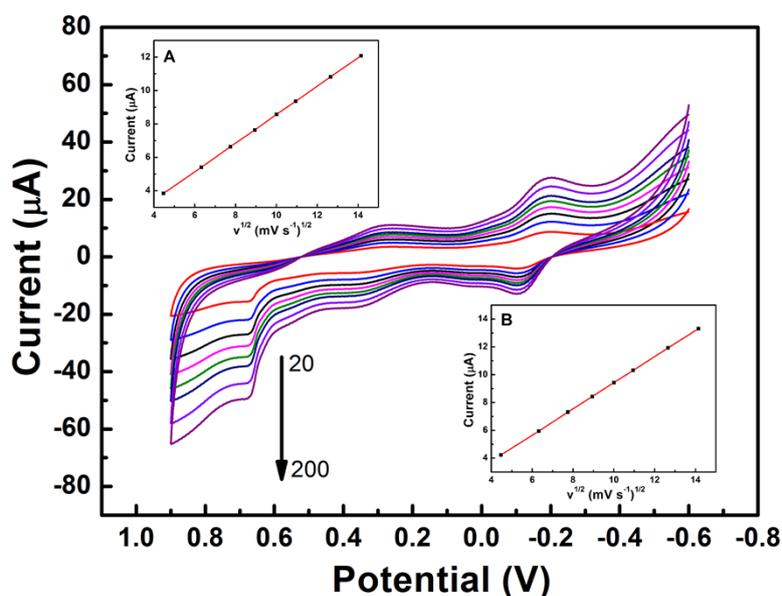
**Fig. S4.** CV of immunosensing probes at different scan rates of 20, 40, 60, 80, 100, 120, 160, 200  $\text{mV s}^{-1}$  in 0.1 M PBS (pH=6.0). Insets showed the anodic peak currents of (A) CEA and (B) AFP proportional to the square root of scan rates.
