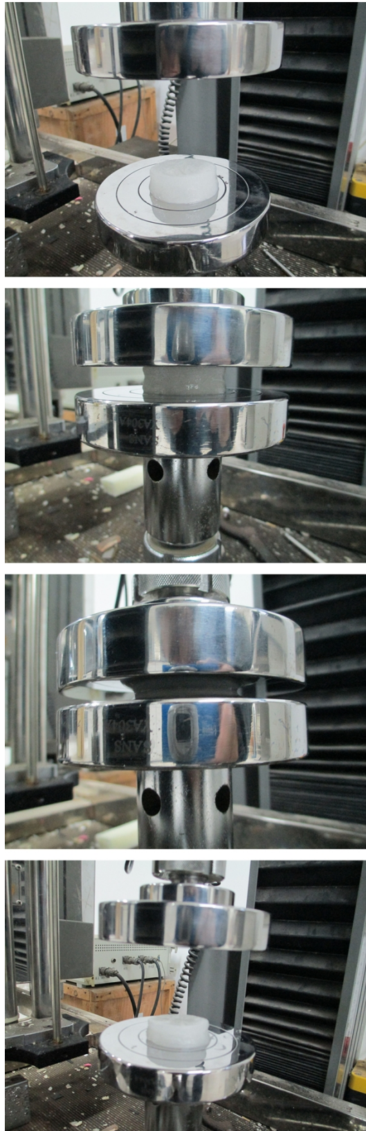
Fig. S1 Photographs of SP3 hydrogel formed at -20\text{ }^{\circ}\text{C} during the compression test.
