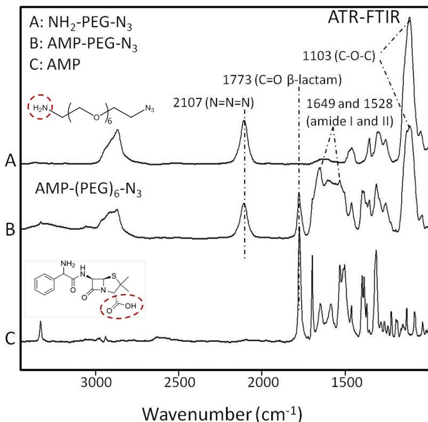
Figure S-1: ATR-FTIR spectra of A – NH<sub>2</sub>-PEG-N<sub>3</sub> (Sigma-Aldrich); B – AMP-PEG-N<sub>3</sub>; and C – AMP reference (reaction sites of A and C are circled).
