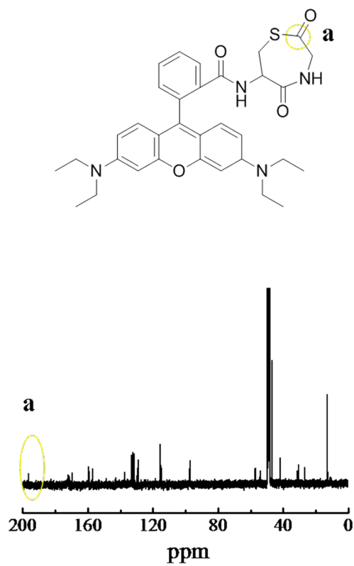
Fig. S10. ^{13}\text{C} NMR spectrum for Rho-Cys-Gly-thiolactone in \text{CD}_3\text{OD}
