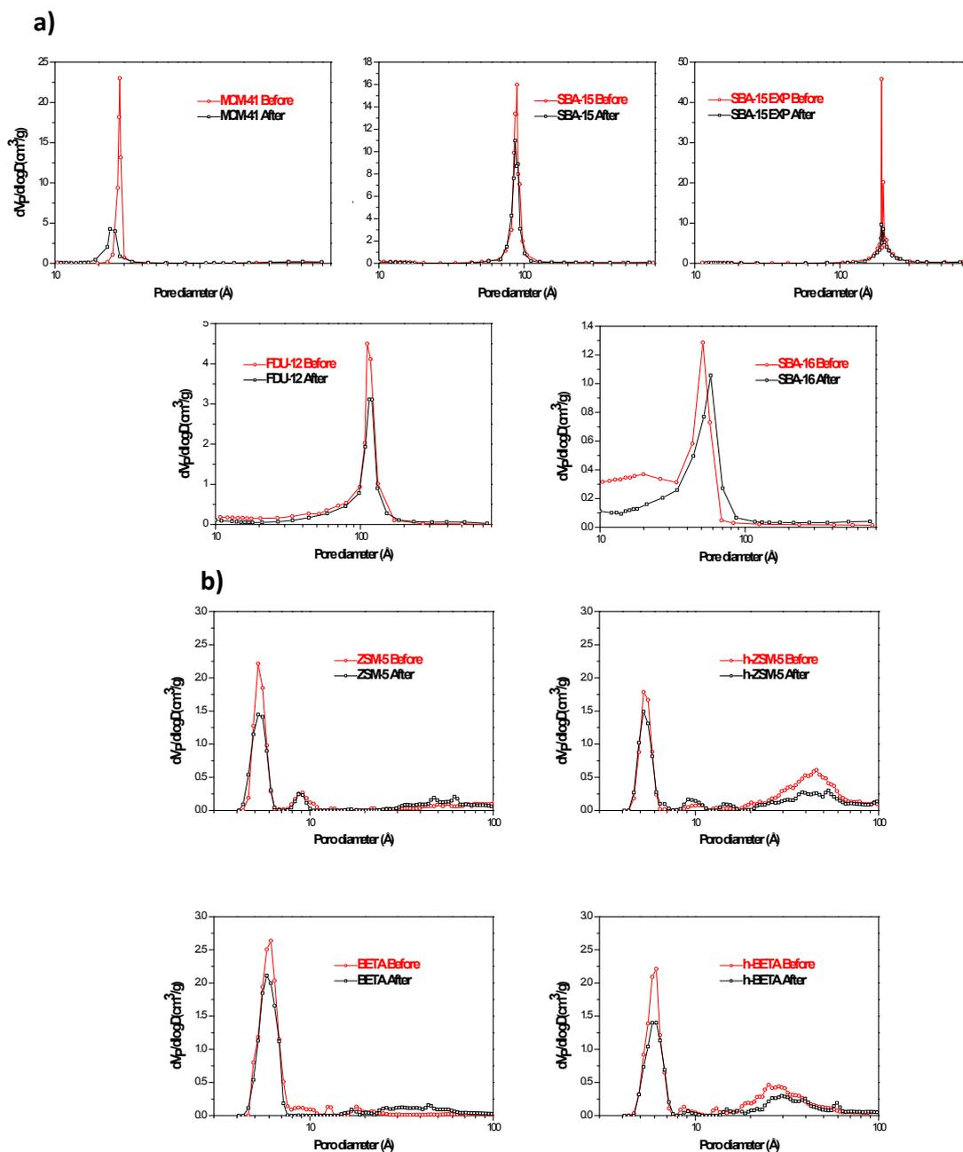
**Figure S5.** a) Pore size distribution obtained by N<sub>2</sub> adsorption-desorption for mesoporous materials (MCM-41, SBA-15, SBA-15 EXP, FDU-12 and SBA-16), and b) by Ar adsorption-desorption isotherms for zeolitic materials (ZSM-5, h-ZSM-5, BETA and h-BETA) before and after drug loading,
