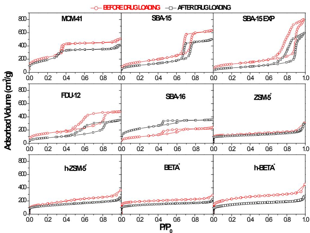
**Figure S4:** N<sub>2</sub> adsorption isotherms for mesoporous materials (MCM-41, SBA-15, SBA-15 EXP, FDU-12 and SBA-16), and Ar adsorption isotherms for zeolitic materials (ZSM-5, h-ZSM-5, BETA and h-BETA) before and after drug loading.
