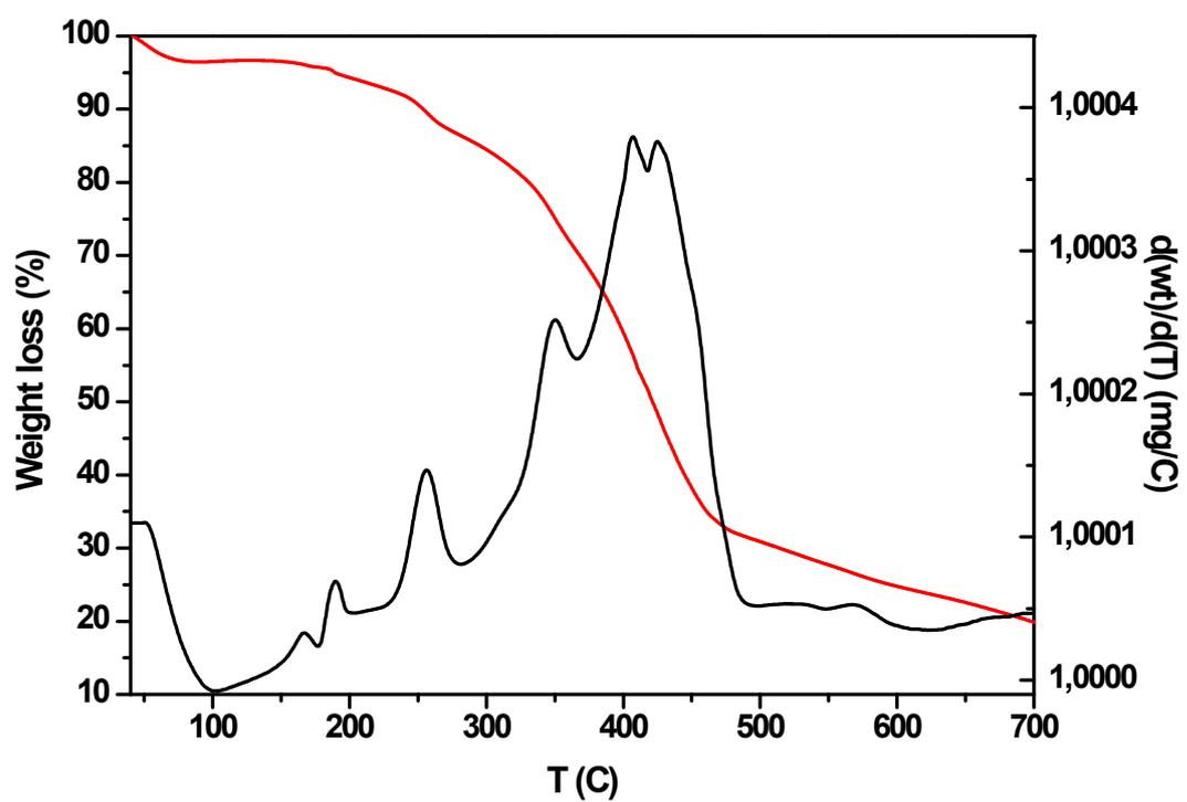
**Figure S1:** Pure methylprednisolone hemisuccinate thermogravimetric analysis (TGA).
