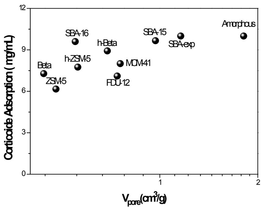
**Figure S6:** Effect of the pore volume on drug loading efficiency.
