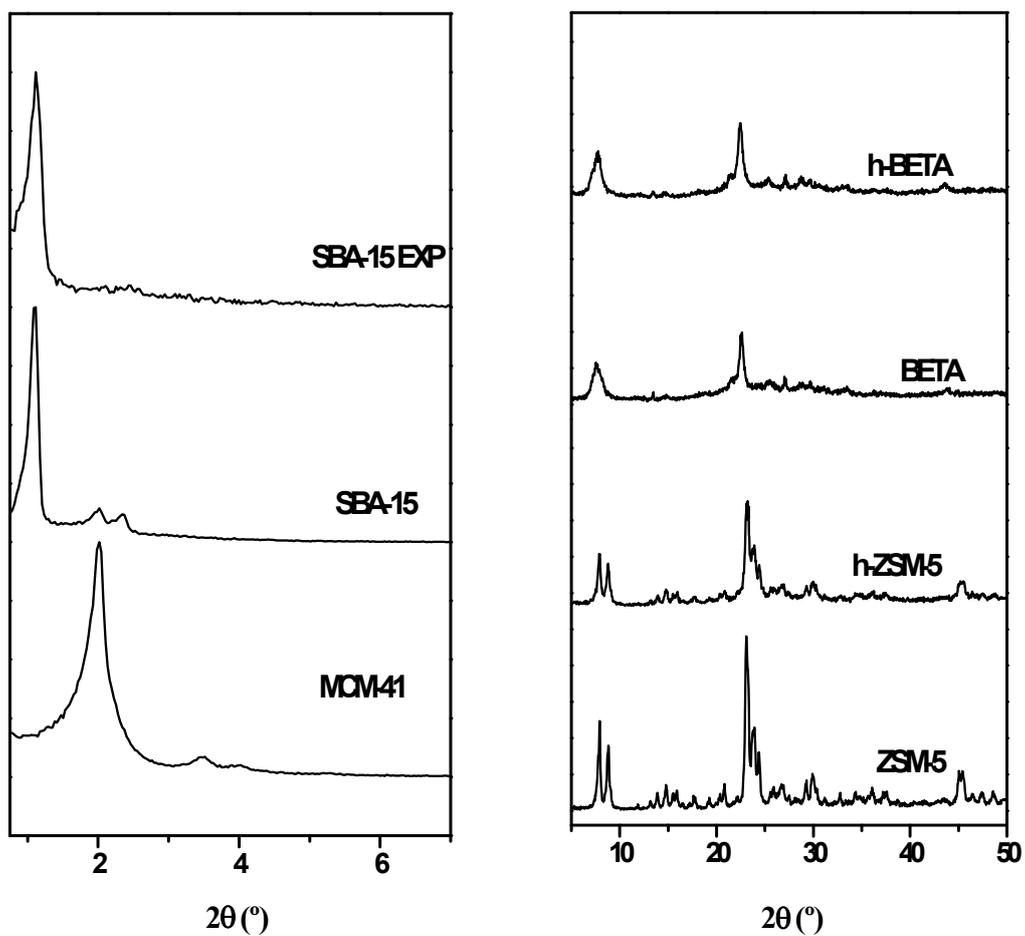
**Figure S3:** XRD patterns at low-angle region of mesoporous materials (MCM-41, SBA-15, SBA-15 EXP), and XRD patterns at wide-angle region of zeolitic materials (ZSM-5, h-ZSM-5, Beta and h-Beta).
