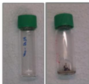
**Figure S5.** Pictures of aldehyde-terminated (right side) and hydroxyl-terminated (left side) copolymer after the Tollens' test
