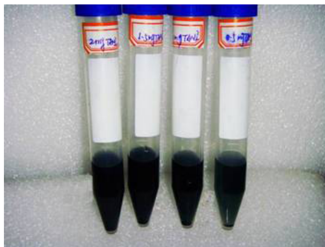
Fig. S4 Photograph of 2 mg, 1.5 mg, 1 mg and 0.5 mg TANI dissolved in 4 ml glacial acetic acid. A small amount of HAc-TANI-ES precipitated out of all four samples, indicating that HAc-TANI-ES has slightly lower solubility in glacial acetic acid.
