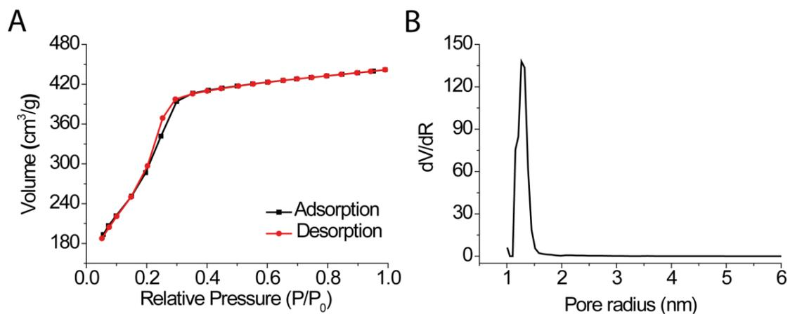
**Figure S2.** (A) N<sub>2</sub> adsorption-desorption isotherms and (B) Pore size distribution, of the MP-SiO<sub>2</sub> NPs. The surface area is 1057 m<sup>2</sup>/g, and the pore diameter corresponds to ~2.8 nm.
