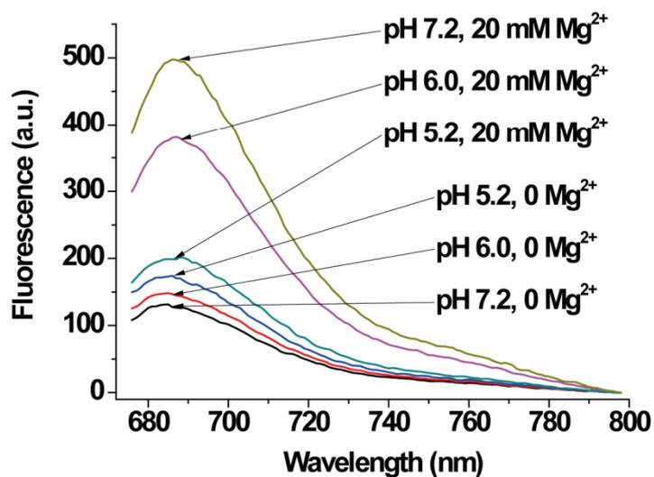
**Figure S3.** The background fluorescence spectra corresponding to the release of  $\text{MB}^+$  from the  $\text{MP-SiO}_2$  NPs without added  $\text{Mg}^{2+}$  ions at different pH values. For comparison the fluorescence spectra of the released  $\text{MB}^+$  in the presence of add 20 mM  $\text{Mg}^{2+}$  ions, at different pH values are shown. All spectra were recorded after fixed a time-interval of 60 minutes of release.
