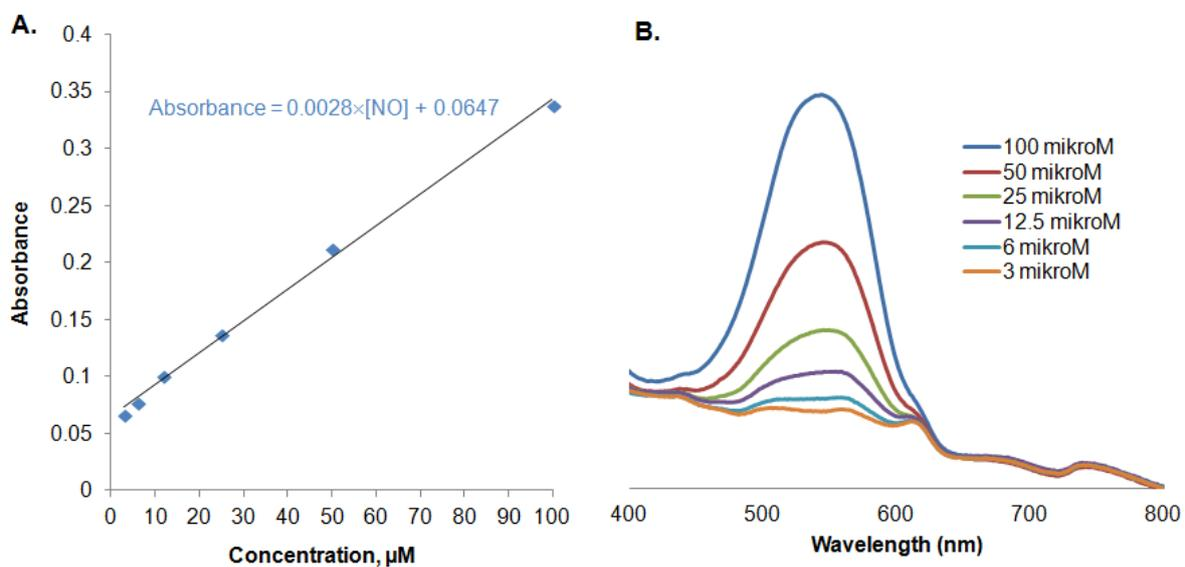
**Figure S7.** Calibration curve (A) and UV-Vis absorption (B) of the azo dye generated in the Griess assay at different concentration of nitric oxide.
