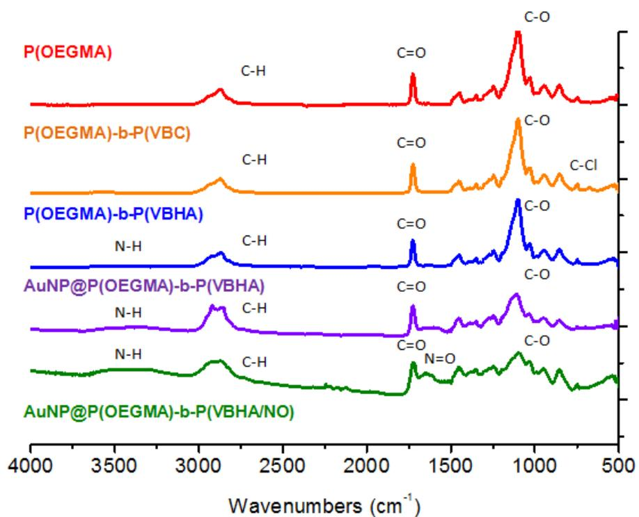
Figure S3. ATR-FTIR of block copolymers and their hybrid gold nanoparticles (AuNP).
