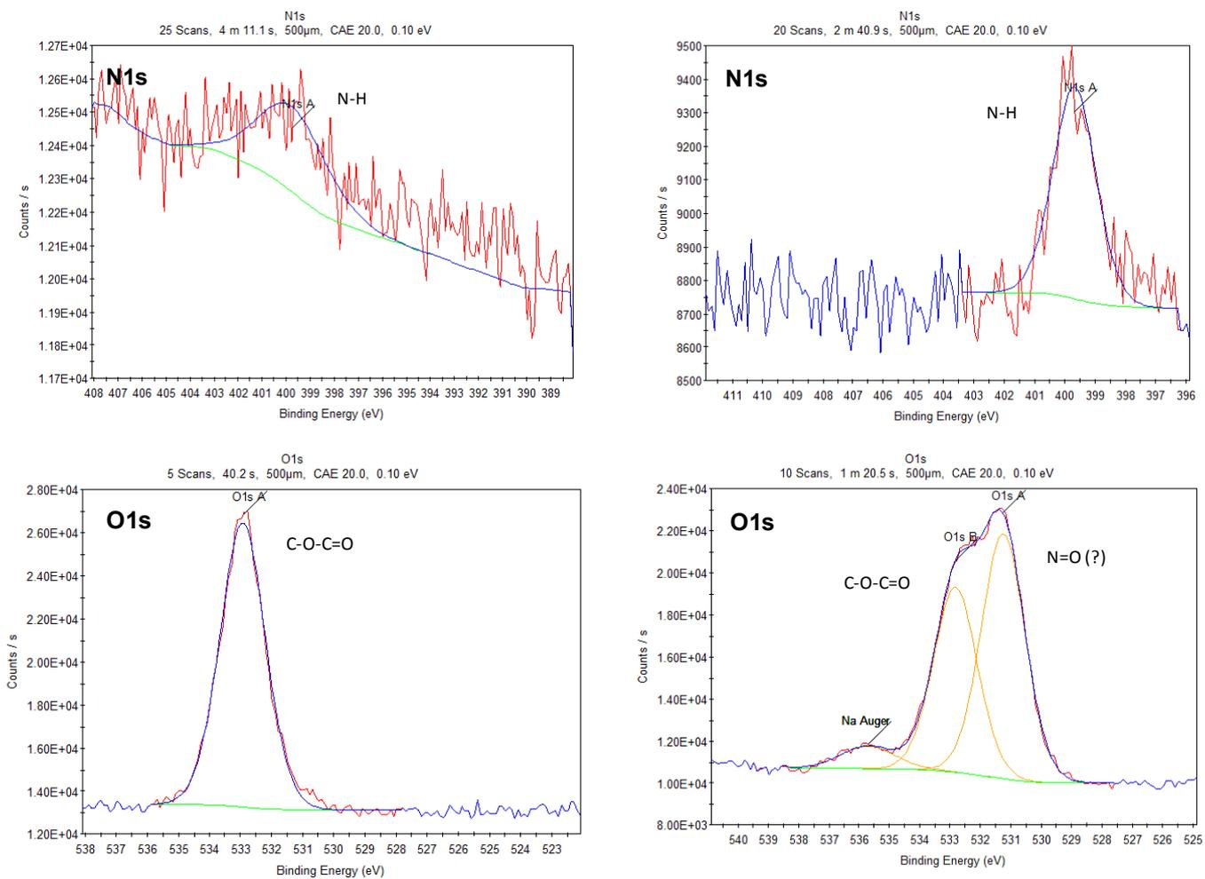
**Figure S5.** Carbon (C1s), nitrogen (N1s) and oxygen (O1s) peaks from the XPS analysis of polymer/gold hybrid nanoparticles AuNP@P(OEGMA)-*b*-P(VBHA) before and after NO conjugation.
