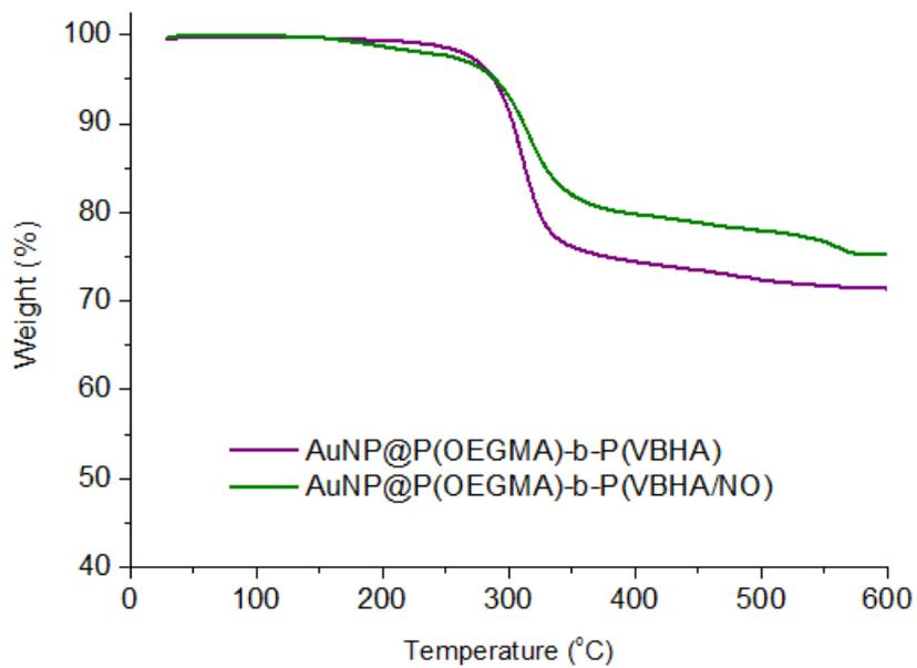
**Figure S6.** TGA of polymer/gold hybrid nanoparticles AuNP@P(OEGMA)-*b*-P(VBHA) before and after NO conjugation. Samples were pre-dried before measurement that potentially releases the nitric oxide gas.
