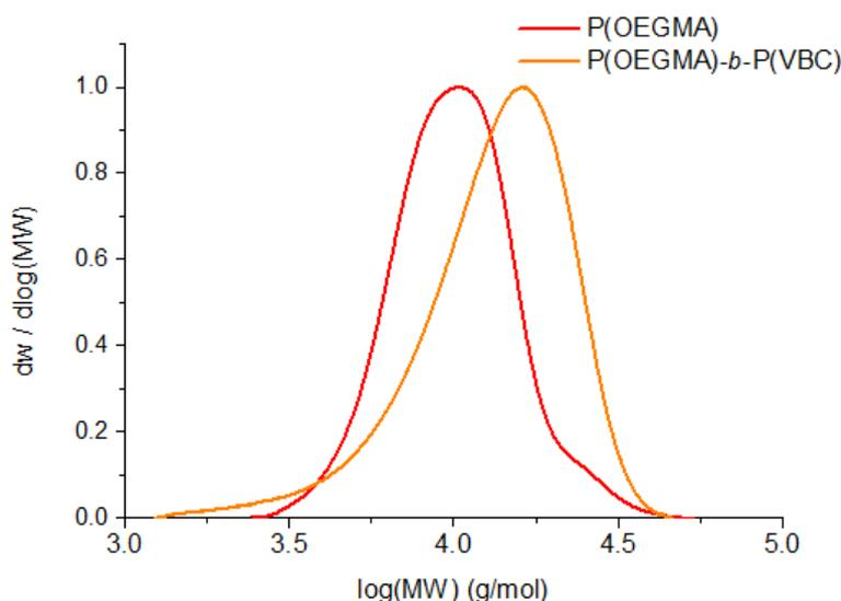
**Figure S1.** SEC of P(OEGMA) and block copolymer P(OEGMA)-*b*-P(VBC).
