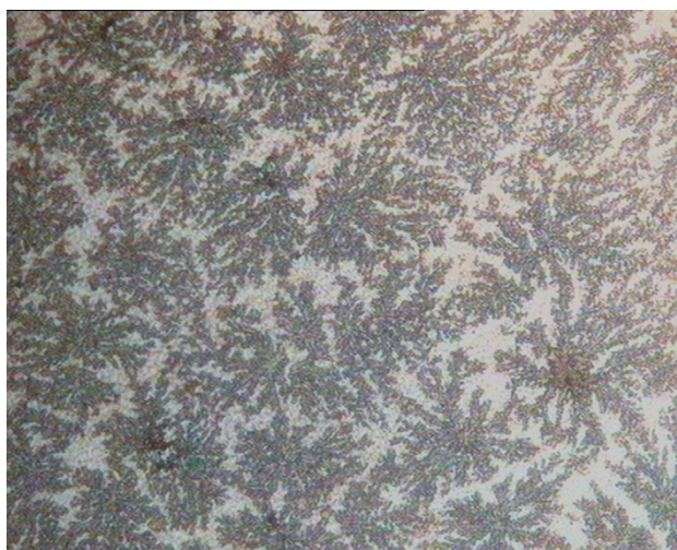
Fig. S3 The morphology of fabricated microgels was observed by transmitting polarized microscope at 1 mg/mL.
