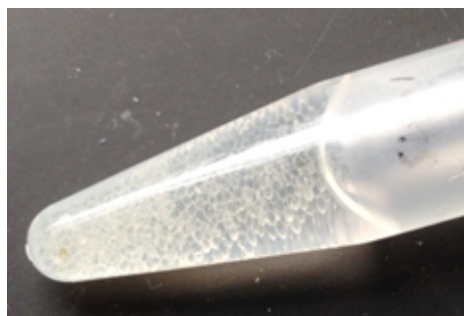
Figure S5. NOX-P22 immobilization on silica beads. P22-NOX was covalently attached to 0.5mm silica beads and assayed for activity 11 days after attachment. Encapsulated enzymes retained activity after immobilization.
