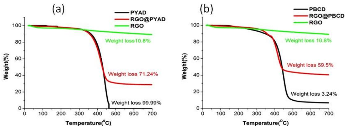
**Figure. S19.** a) TGA curves of RGO, RGO@PYAD and PYAD and b) Thermogravimetric analysis of RGO, RGO@PBCD and PBCD.
