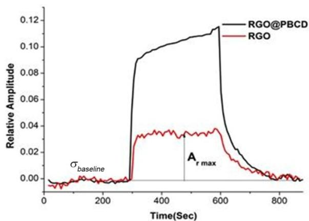
**Figure S22.** Signal to noise ratio of RGO and RGO@PBCD sensors at 400 ppb of benzene.
