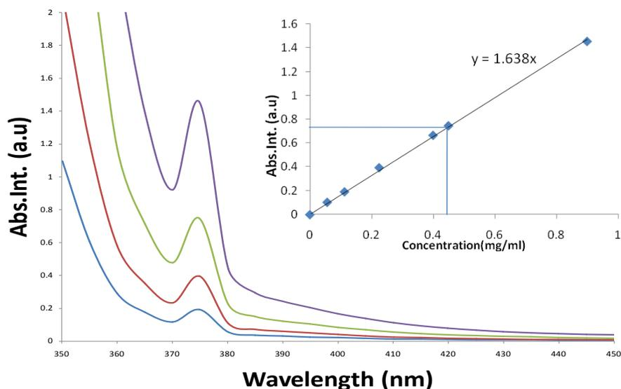
**Figure S20.** UV-vis spectra of PYAD in ethanol concentrations of 0.9 mg/mL (violet curve),  $0.45 \text{ mg}\cdot\text{cm}^{-3}$  (green curve),  $0.225 \text{ mg}\cdot\text{cm}^{-3}$  (red curve),  $0.1156 \text{ mg}\cdot\text{cm}^{-3}$  (blue curve) and Absorbance vs concentration at constant wavelength 286 nm curve following LAMBERT BEER'S law (inset).
