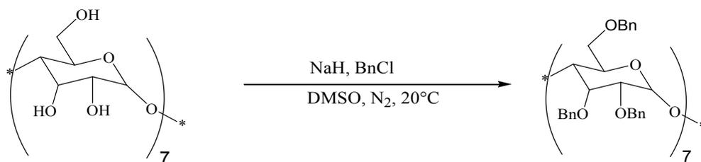
**Figure S8.** Synthesis of perbenzylated cyclodextrin.
