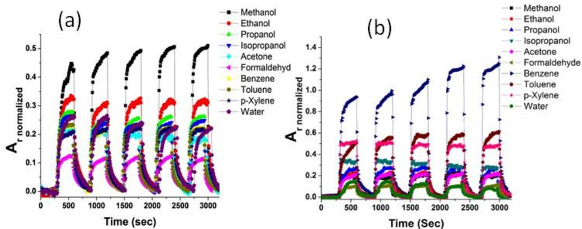
**Figure S21.** Chemo-electrical response of (a) RGO@PYAD-MCD and (b) RGO@PBCD sensor in a set of 10 VOC.
