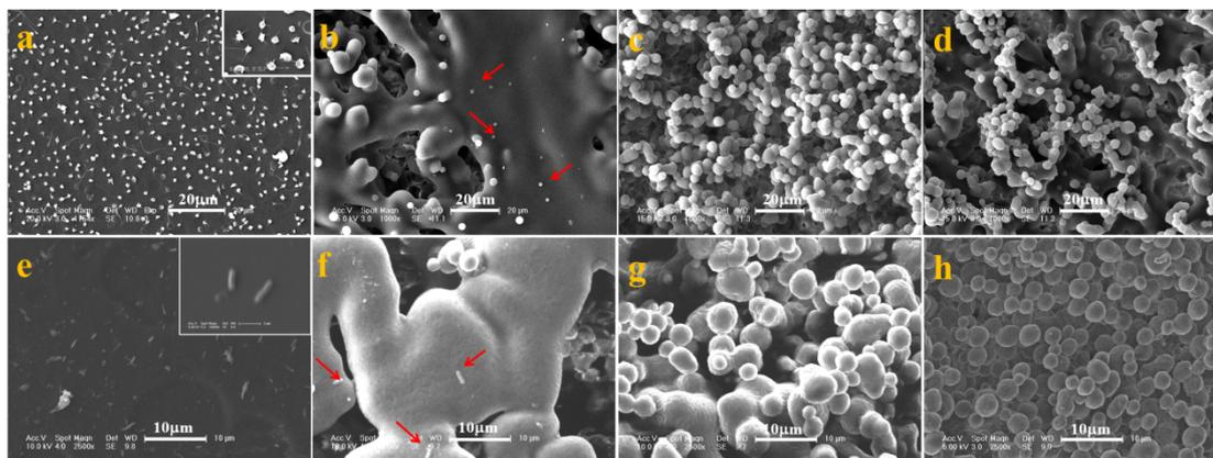
Fig. S4. (a-d) SEM images of platelet adhesion on virgin SEBS, SEBS<sub>1</sub>, SEBS<sub>2</sub> and SEBS<sub>3</sub>, respectively; (e-h) SEM images of bacterial adhesion on virgin SEBS, SEBS<sub>1</sub>, SEBS<sub>2</sub> and SEBS<sub>3</sub>, respectively.
