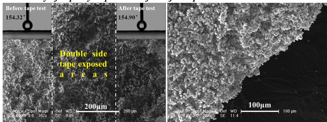
Fig. S2. SEM images of superhydrophobic surface that were exposed to double side tape (white boxes indicate the exposed areas) and the cross section of superhydrophobic SEBS films.
