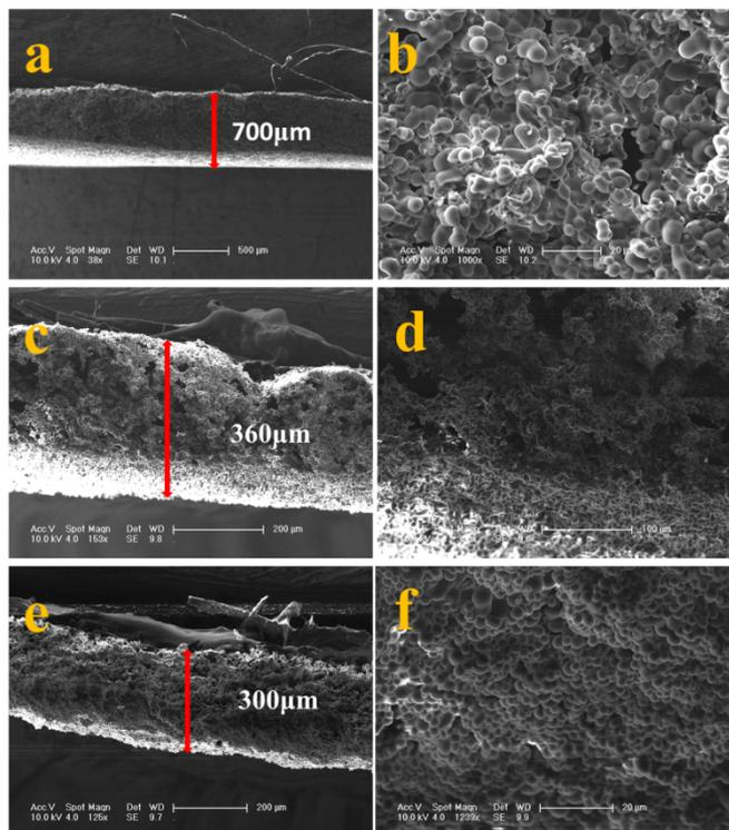
Fig. S5. (a, c, e) SEM images of SEBS films (cross section) with various thickness and (b, d, f) the surface morphology of corresponding samples.
