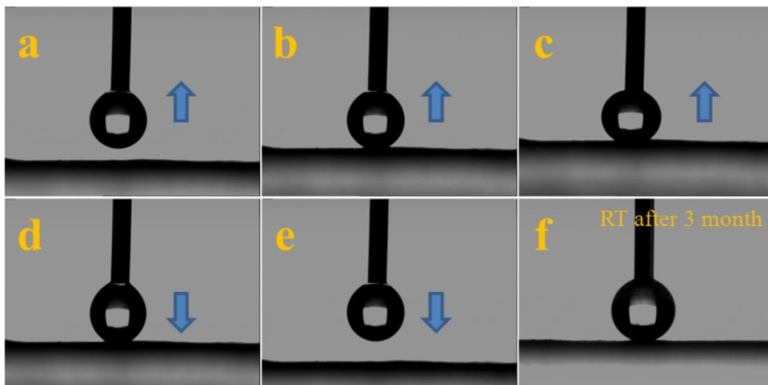
Fig. S1. Superhydrophobic properties of surface and stability of superhydrophobic surface at room temperature. a-e) The approach and departure process of an 2  $\mu\text{l}$  water droplet from the SEBS<sub>3</sub> surface, the arrows represent the moving direction of substrate, f) The water contact angle on surface of SEBS<sub>3</sub> film remains higher than 150° after three months at room temperature.
