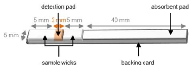
Figure 1: Schematic representation of an immunochromatographic strip.
