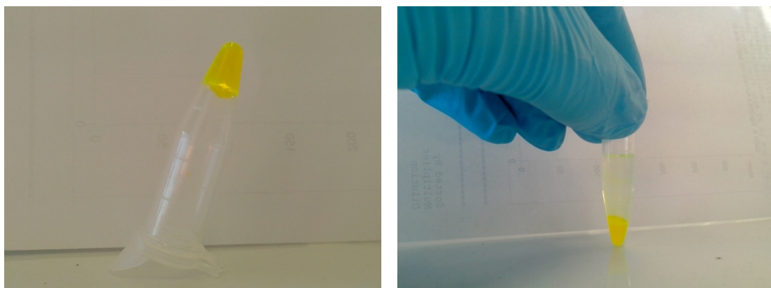
Figure S3. Pictures of the self-assembled hydrogel of MBG-1 encapsulated with 0.1% w/v fluorescein sodium.
