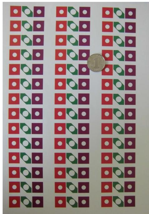
**Fig. S1A** Wax-printed 3D PEC origami device on a paper sheet (A4) before baking.
