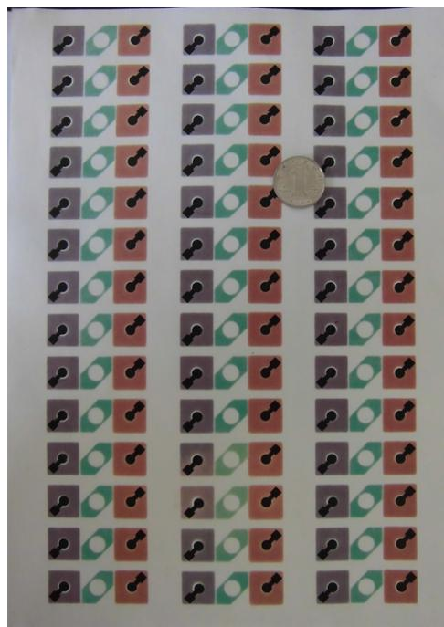
**Fig. S1D** 3D PEC origami device on a paper sheet (A4) after screen-printing of carbon working electrodes on one surface of paper.
