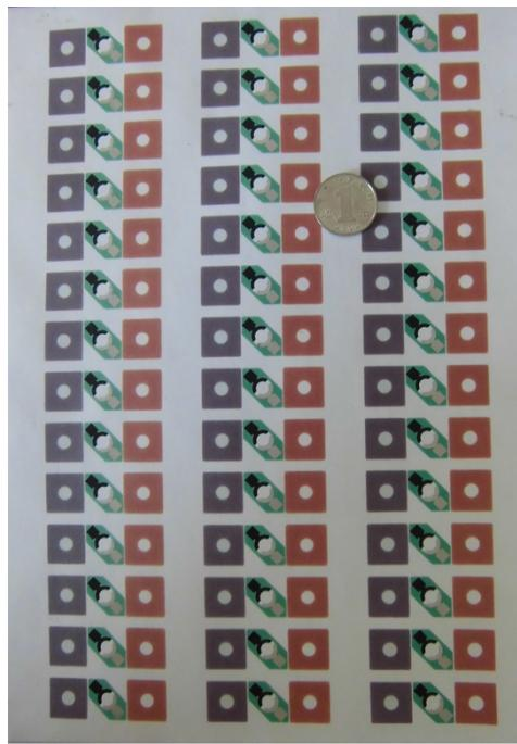
**Fig. S1C** 3D PEC origami device on a paper sheet (A4) after screen-printing of Ag/AgCl auxiliary electrode and carbon counter electrode on one surface of paper.
