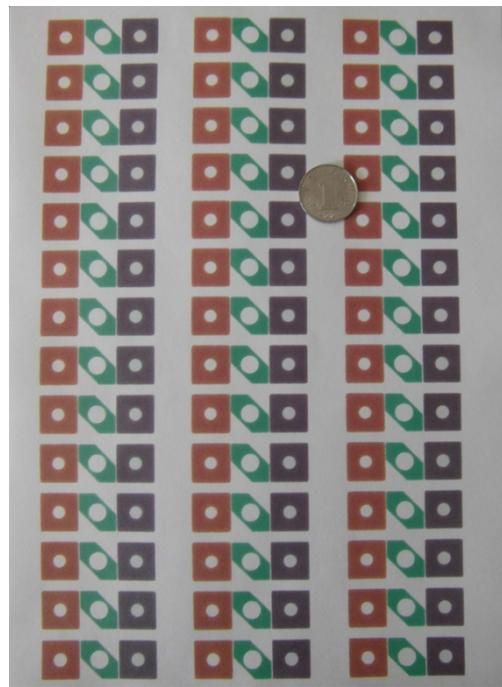
**Fig. S1B** Wax-printed 3D PEC origami device on a paper sheet (A4) after baking.
