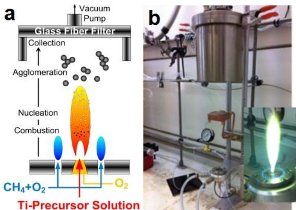
**Figure S2.** (a) Schematic and (b) photograph of flame spray pyrolysis burner at the Nanotechnology Research Laboratory, ANU, utilized for the synthesis and collection of TiO<sub>2</sub> nanostructured powders.
