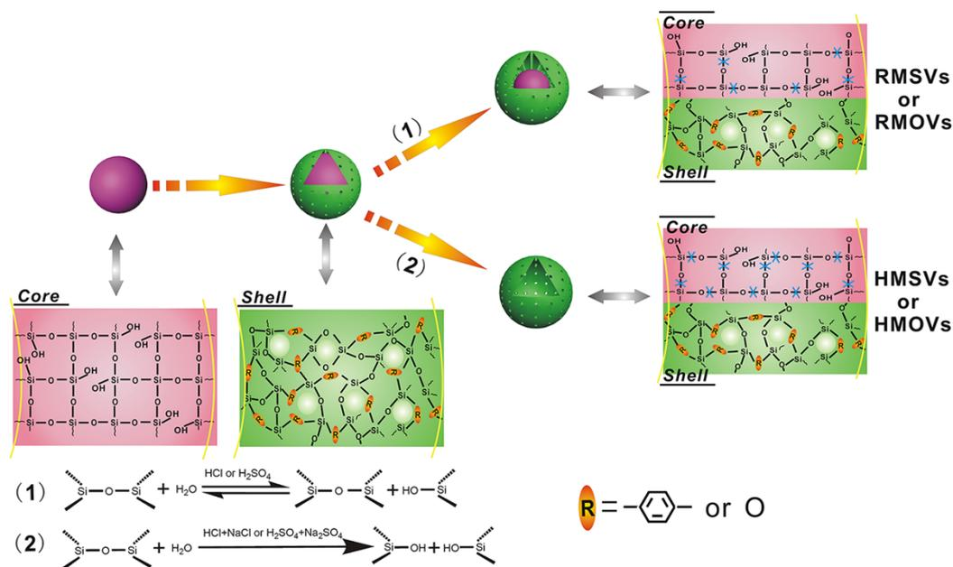
**Figure S1.** Schematic illustration of the synthetic procedure for R/HMSVs and R/HMOVs employing the acid etchants such as HCl, H<sub>2</sub>SO<sub>4</sub> and NaCl, Na<sub>2</sub>SO<sub>4</sub>. The R moiety within the shell framework is phenylene (aromatic) group or oxygen.
