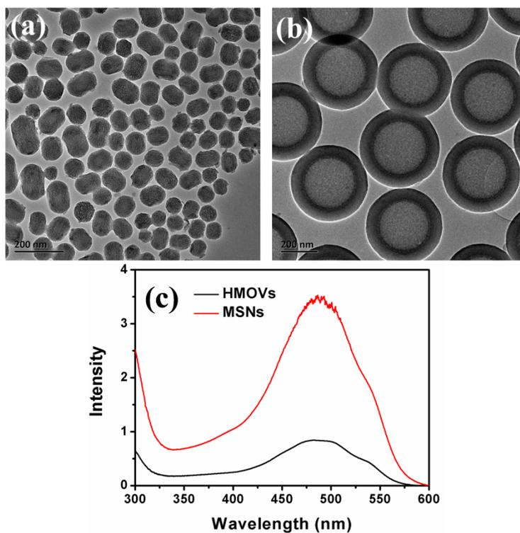
**Figure S3.** TEM images of MSNs (a) and HMOVs (b). UV-Vis spectra of DOX supernatant solution after loaded in MSNs (a) and HMOVs (b).
