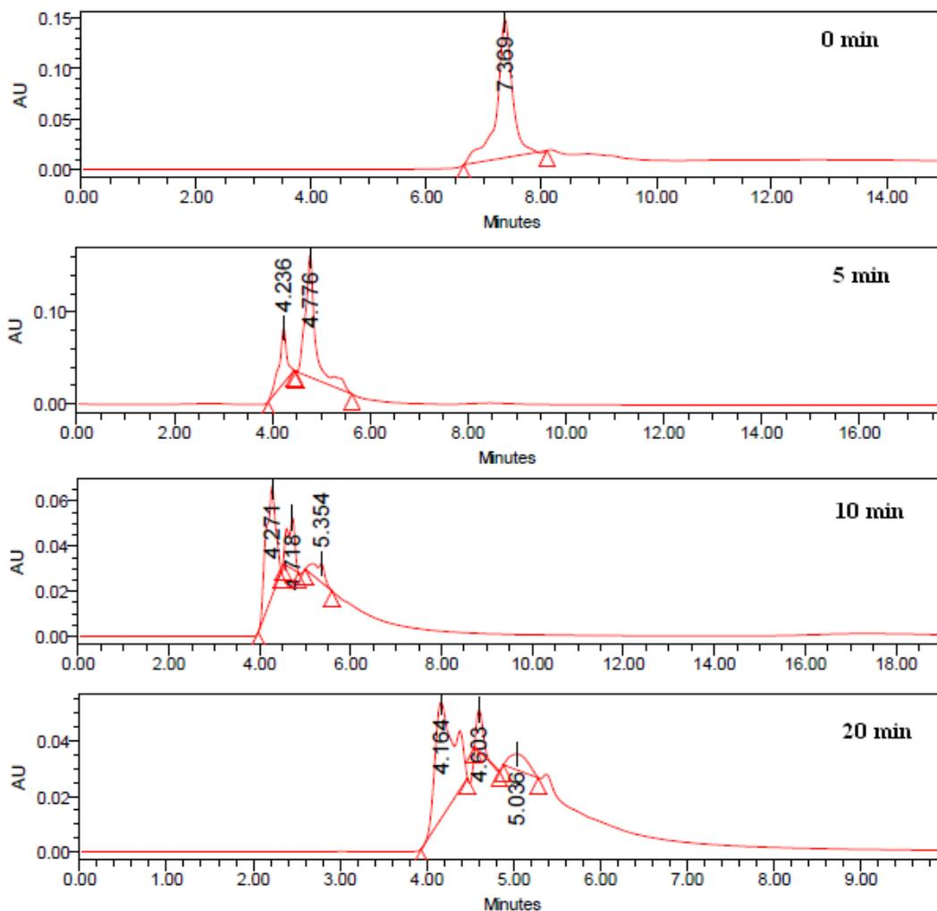
**Figure S1:** HPLC profile of ONB-CC under soft UV irradiation ( $\geq 365$  nm) .
