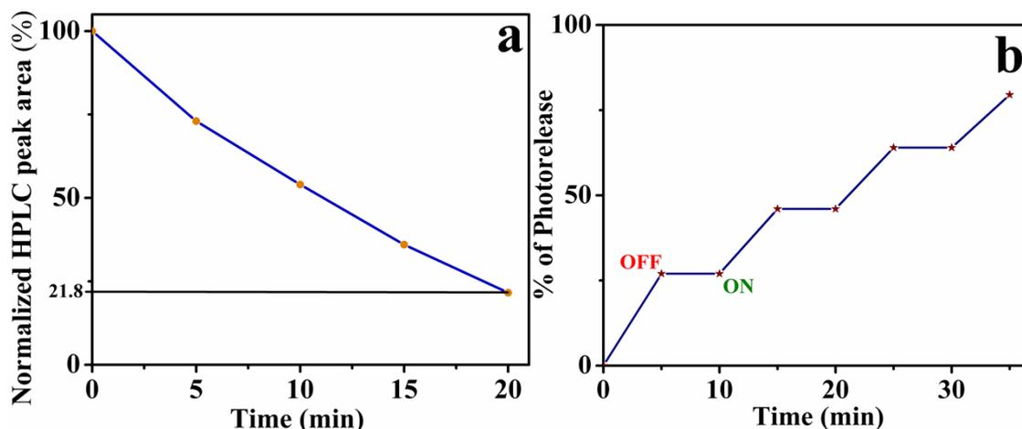
**Figure S2:** (a) Time course for the photorelease of ONB-CC soft UV irradiation ( $\geq 365$  nm) (b) Control over the release under bright and dark conditions. “On” indicates the beginning of light irradiation and the “OFF” indicates the ending of light irradiation
