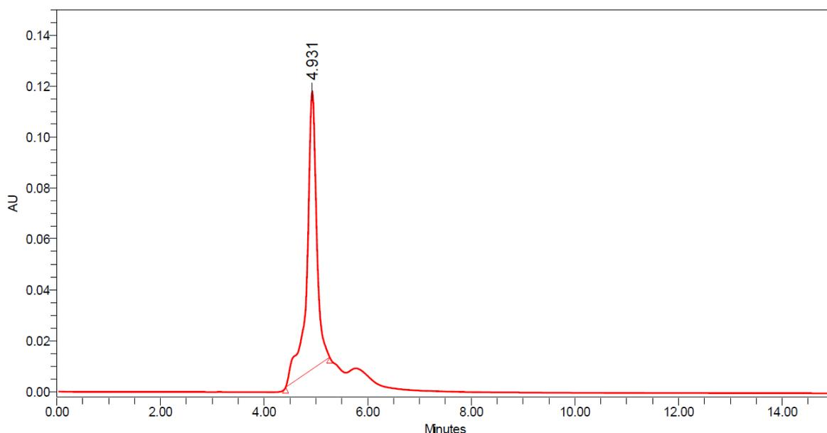
RP-HPLC profile of biotin tagged ONB-CC using mobile phase acetonitrile/water (50/50 v/v), at a flow rate of 1mL/min (detection: UV 254 nm)
