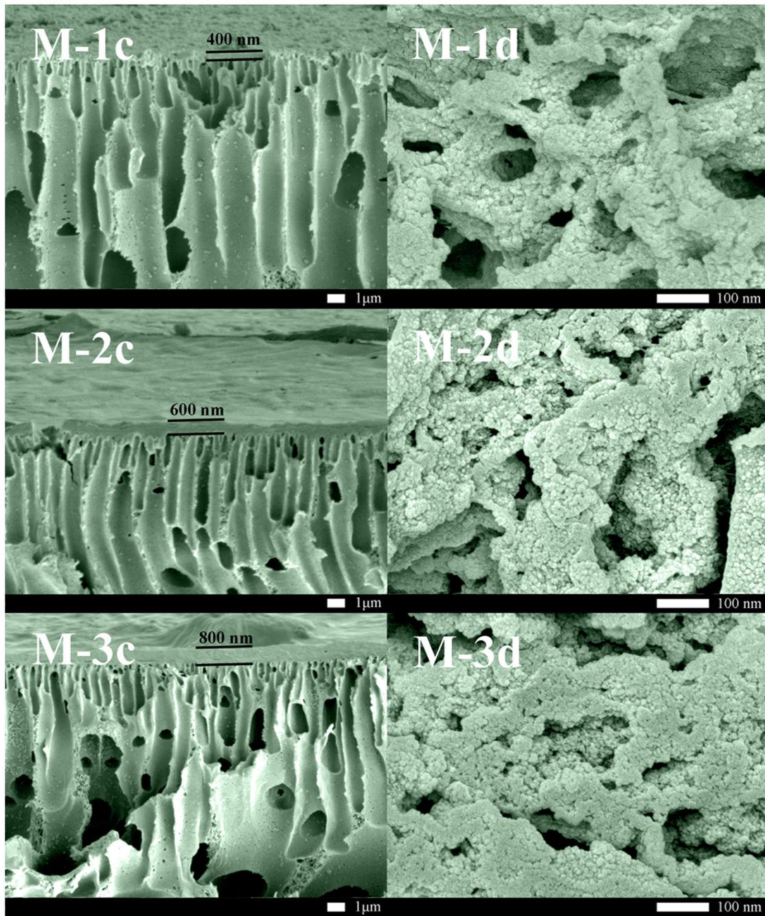
**Figure S2.** Cross-sectional SEM images of the WHP/QC LBL (M-1, M-2, M-3) membranes. (c,  $\times 3000$ ; d,  $\times 80000$ )
