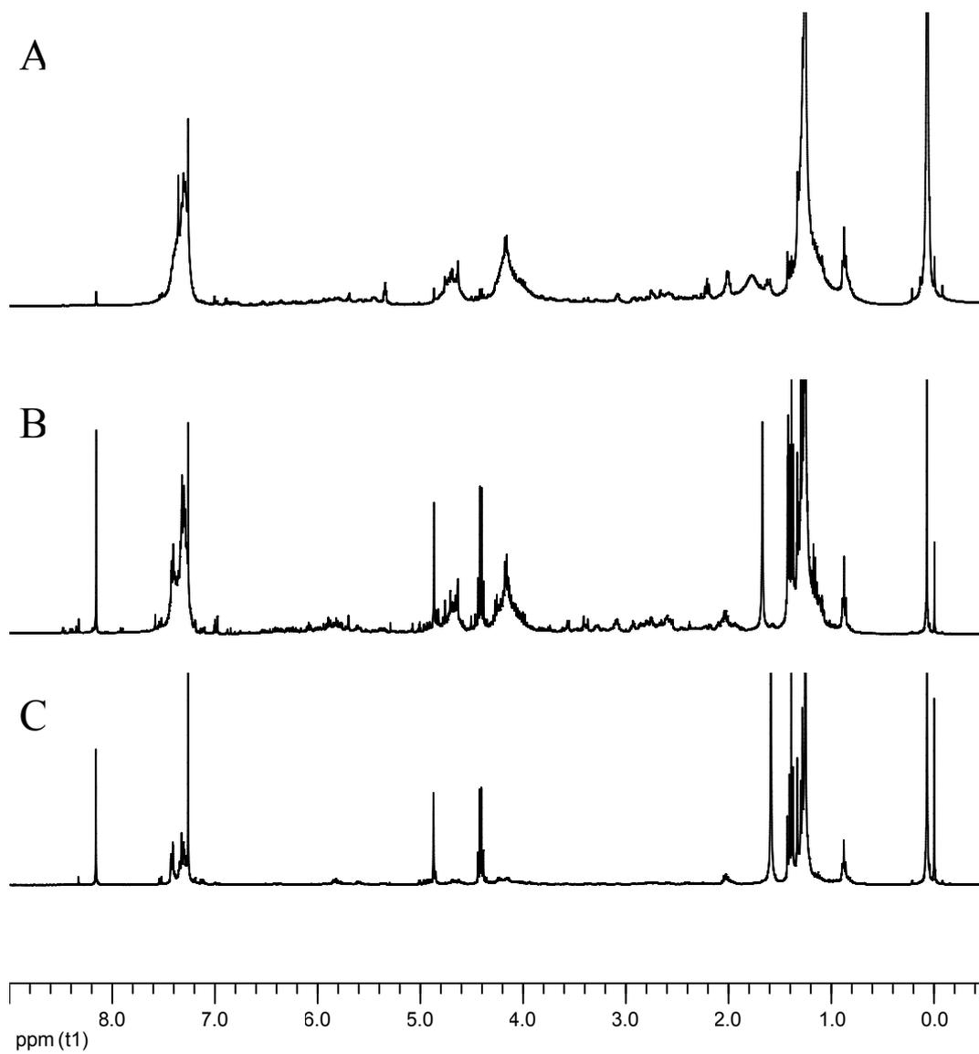
Figure S15. Comparison of  $^1\text{H}$  NMR spectra of Bergman cyclization products. A) polymer, B) oligomer, C) monomer (compound **5**).
