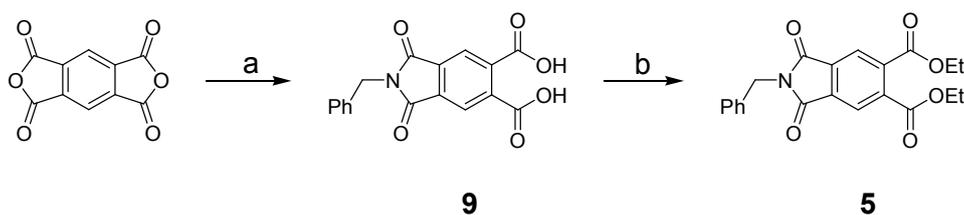
Scheme S3. Synthesis of model compound **9**. (a) benzyl amine, acetic acid, reflux; (b) dichloromethane, ethanol, DCC, DMAP, room temperature.
