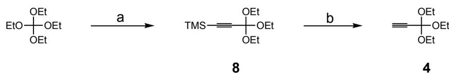
Scheme S2. Synthesis of compounds **4**. (a) TMSA, EtMgBr, diethyl ether; (b) TBAF, THF, 15 min.
