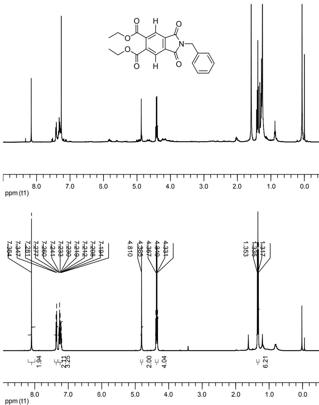
Figure S14. Comparison of  $^1\text{H}$  NMR spectra of compound **5** obtained from Bergman cyclization (upper panel) and from 1,2,4,5-Benzenetetracarboxylic anhydride (lower panel)
