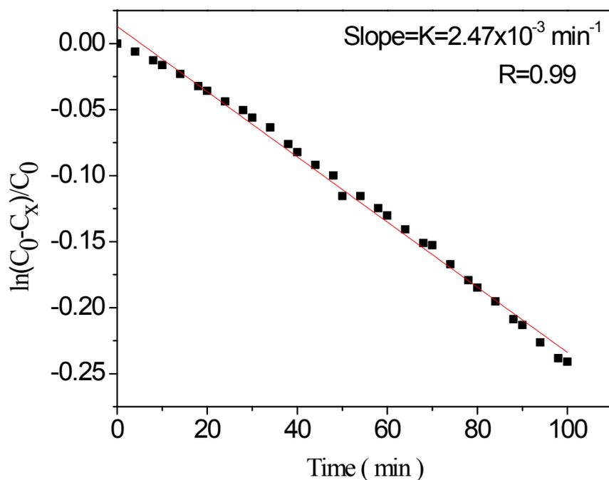
Figure S3. Rate profile for the Bergman cyclization of enediyne **2** in methanol. The line was drawn by least-squares fitting in single exponential equation.  $C_0$  is the initial concentration of enediyne while  $C_x$  is the concentration of enediyne at the given time.
