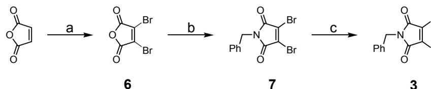
Scheme S1. Synthesis of compounds **3**. (a) Br<sub>2</sub>, AlCl<sub>3</sub>, 120 °C, 16 h; (b) PhCH<sub>2</sub>NH<sub>2</sub>, acetic acid, 22 h; (c) NaI, acetic acid, 5 h.
