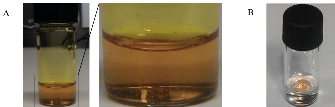
Figure S3. A) UV irradiation prior to electrospinning caused precipitation of AAB from the aqueous IC solution. B) AAB suspension in water.
