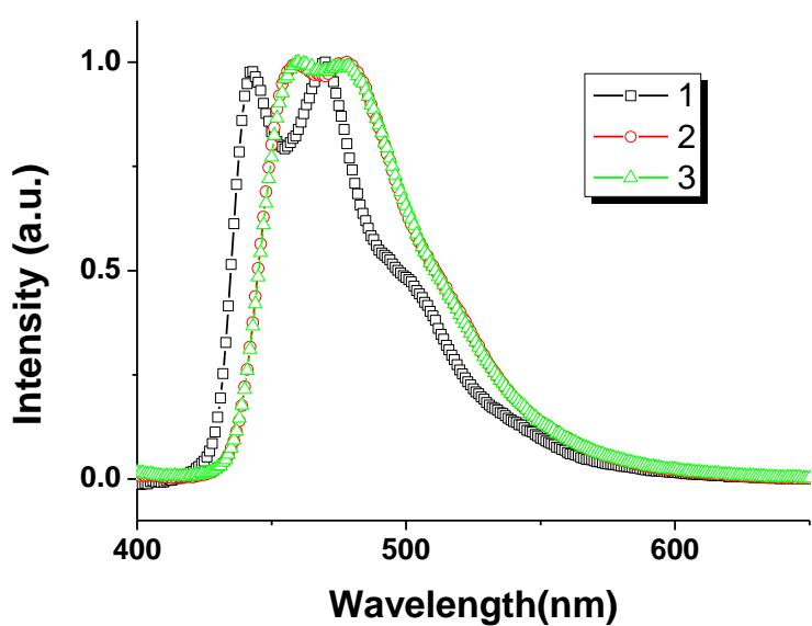
**Figure S13.** Emission spectra of **1**, **2** and **3** in the solid state at 298K (10 %wt- PMMA film).
