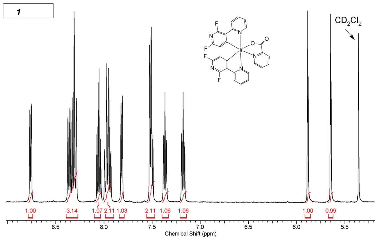
**Figure S2.**  $^1\text{H}$  NMR of **1** in CD<sub>2</sub>Cl<sub>2</sub>.
