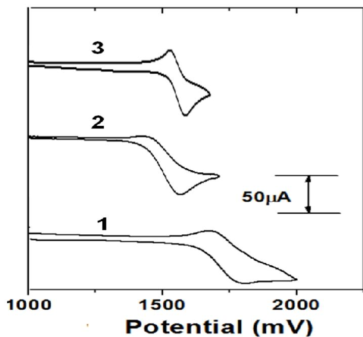
**Figure S14.** Comparison of oxidation potentials (vs Ag/AgCl in CH<sub>3</sub>CN) of **1**, **2** and **3** ( oxidation potential FeCp<sub>2</sub>/FeCp<sub>2</sub><sup>+</sup> =0.45 V)
