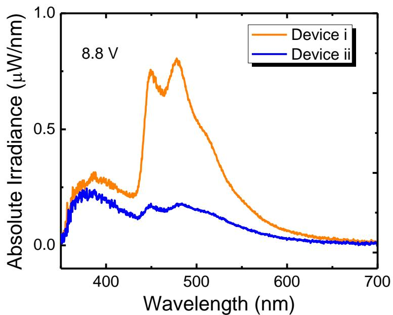
**Figure S15.** EL spectra of **1** using different hole-transporting and host materials. Device **i**: ITO(120 nm)/MoO<sub>3</sub>(1 nm)/CBP(35 nm)/CDBP-doped with 20 wt% of **1**(15 nm)/TPBi(65 nm) /LiF (1 nm)/Al (100 nm); Device **ii**: ITO(120 nm)/MoO<sub>3</sub>(1 nm)/CBP(35 nm)/CBP-doped with 20 wt% of **1**(15 nm)/TPBi(65 nm) /LiF (1 nm)/Al (100 nm).
