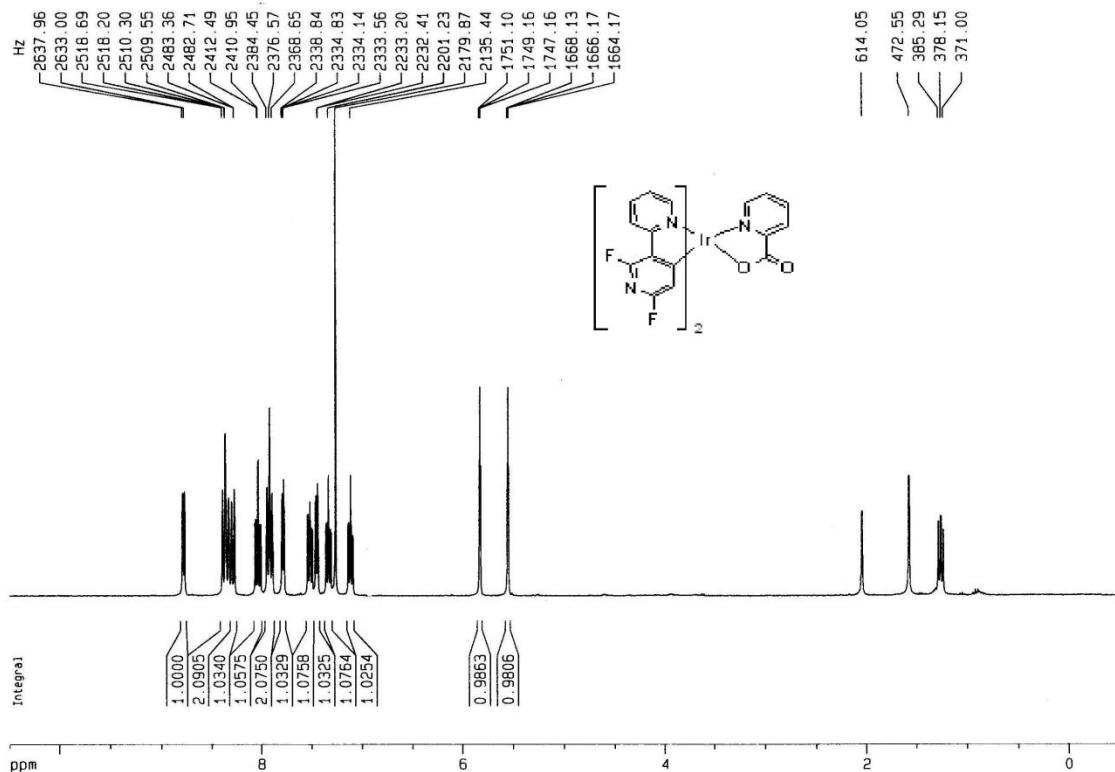
**Figure S3.** <sup>1</sup>H NMR of **1** in CDCl<sub>3</sub>; compound **1** was obtained by using different reaction conditions (in the presence of NEt<sub>3</sub> at 120 °C ; refluxing toluene).
