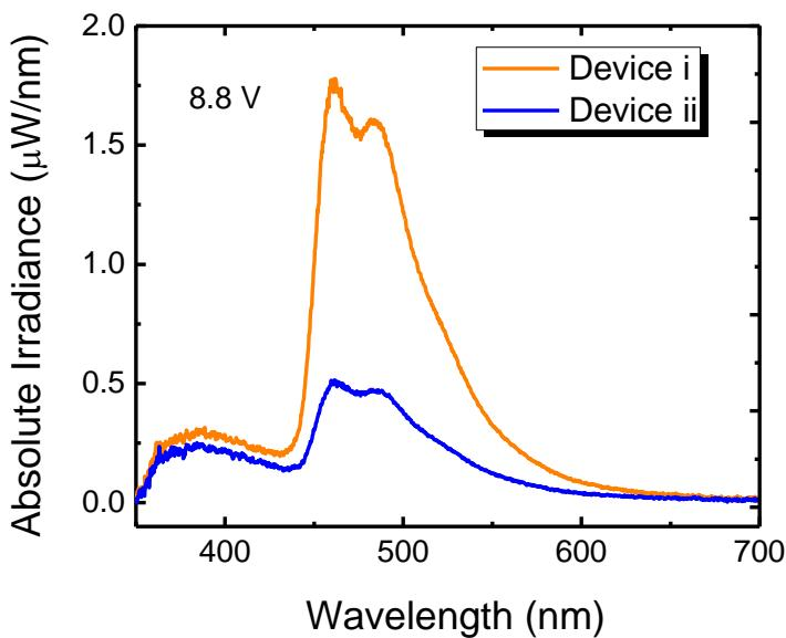
**Figure S16.** EL spectra of **2** using different hole-transporting and host materials. Device **i**: ITO(120 nm)/MoO<sub>3</sub>(1 nm)/CBP(35 nm)/CDBP-doped with 20 wt% of **2**(15 nm)/TPBi(65 nm) /LiF (1 nm)/Al (100 nm); Device **ii**: ITO(120 nm)/MoO<sub>3</sub>(1 nm)/CBP(35 nm)/CBP-doped with 20 wt% of **2**(15 nm)/TPBi(65 nm) /LiF (1 nm)/Al (100 nm).
