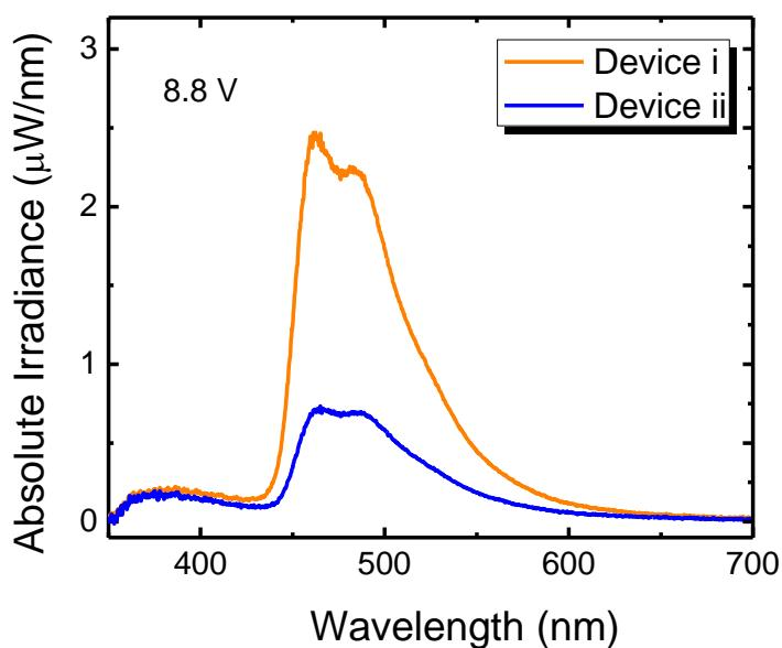
**Figure S17.** EL spectra of **3** using different hole-transporting and host materials. Device **i**: ITO(120 nm)/MoO<sub>3</sub>(1 nm)/CBP(35 nm)/CDBP-doped with 20 wt% of **3**(15 nm)/TPBi(65 nm)/LiF (1 nm)/Al (100 nm); Device **ii**: ITO(120 nm)/MoO<sub>3</sub>(1 nm)/CBP(35 nm)/CBP-doped with 20 wt% of **3**(15 nm)/TPBi(65 nm)/LiF (1 nm)/Al (100 nm).
