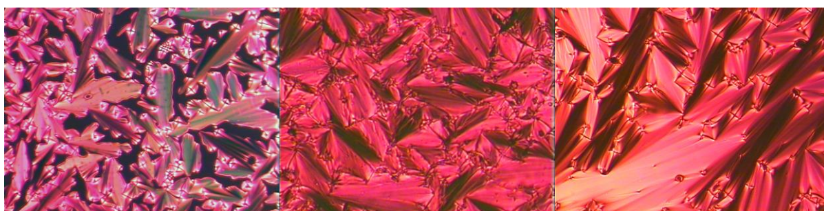
Supporting Figure 4. Optical polarising microscopy images 6 (a) at 141 °C and 6-Zn(II) (b) at 141 °C, 6-Ni(II) (c) at 158 °C.
