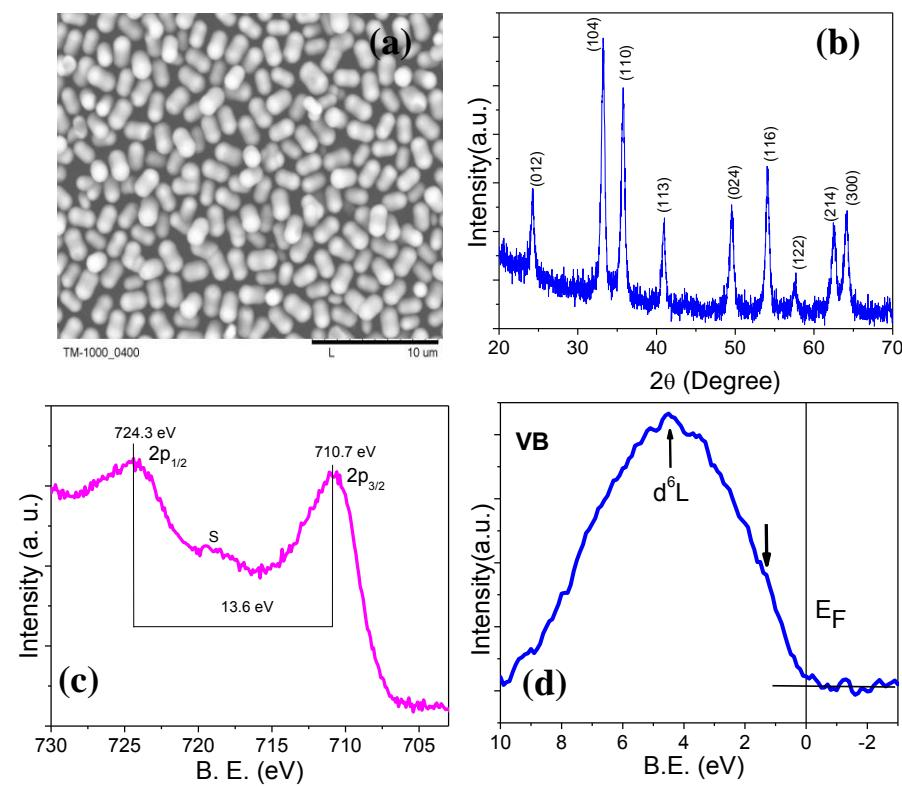
Fig. S1: (a) SEM microstructure, (b) XRD data, (c) Fe 2p spectrum and (d) VB spectrum of synthesized  $\alpha$ -Fe<sub>2</sub>O<sub>3</sub> particle
