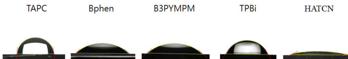
Fig. S1 Distilled water contact angle for TAPC, Bphen, B3PYMPM, TPBi, and HATCN, respectively.
