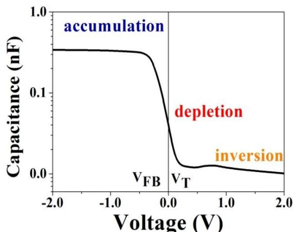
**Figure 1S.** Typical high frequency capacitance vs voltage response of a MIS structure on a p-type semiconductor and corresponding working conditions. Flat band and threshold voltages are indicated too.
