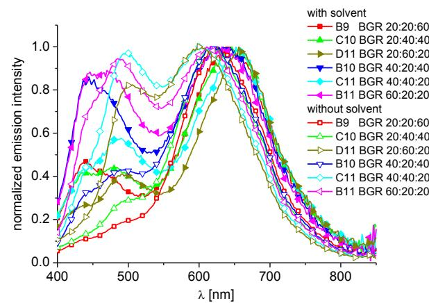
Figure S5. Emission spectra of films B9 – B11, C10, C11 and D11 inkjet-printed with or without solvent (film,  $\lambda_{\text{ex}} = 365 \text{ nm}$ ).
