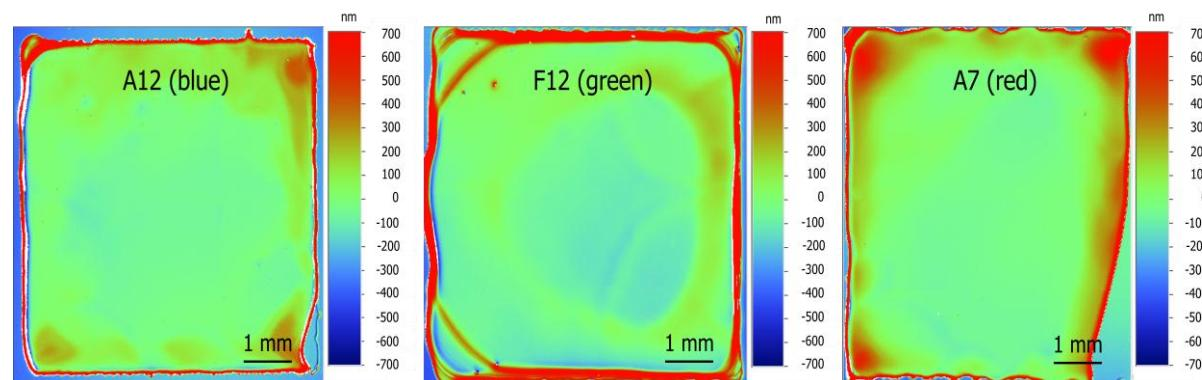
Figure S3. Optical profiler image of films A12, F12 and A7 inkjet-printed with a dot spacing of 90  $\mu$ m using a 5 mg/mL solution of DMF/AcPh (9/1) and a substrate temperature of 50 °C.
