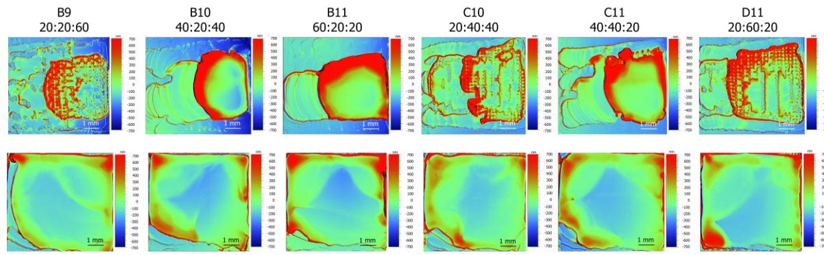
Figure S4. Optical profiler image of films B9 – B11, C10, C11 and D11 inkjet-printed without (first row) and with (second row) one additional layer of solvent.
