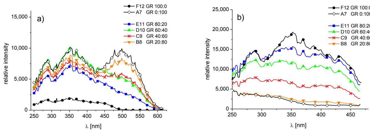
Figure S7. Excitation spectra of A7, B8, C9, D10, E11 and F12 a) (film,  $\lambda_{\text{em}} = 650$  nm); b) (film,  $\lambda_{\text{em}} = 500$  nm).
