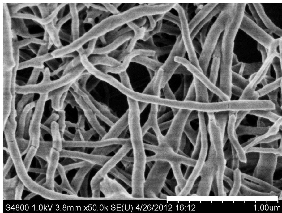
Fig. S6 Enlarged SEM image of **1a** in gel state of PrOH formed by sonication (0.16 W cm<sup>-2</sup>, 40 KHz, 40 °C, 30 min)
