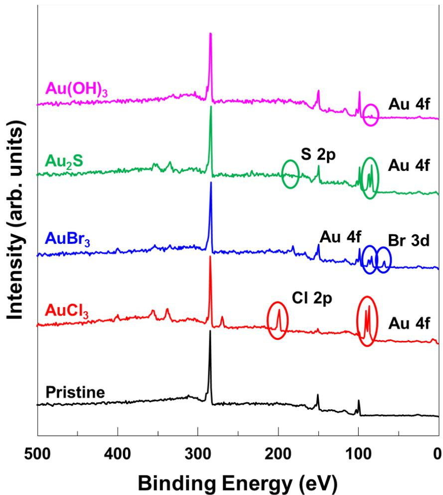
**Figure SI3.** The wide scan of the Au complex doped graphene sheets. Each Au complex doped graphene sheet had anions peak for Cl 2p, Br 3d, S 2p. The Au 4f peak indicated the presence of gold ions on the graphene sheets.
