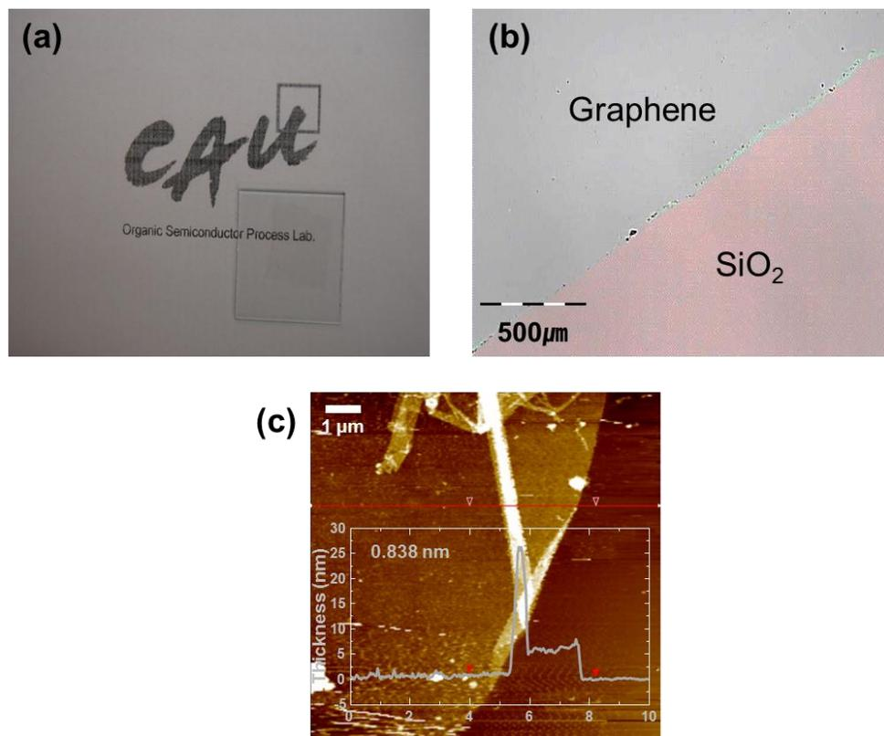
**Figure S11.** a) The photographic image of pristine graphene on a glass substrate. b) The optical microscopic image of transferred pristine graphene on SiO<sub>2</sub> wafer. c) The thickness profile and AFM image of pristine graphene on SiO<sub>2</sub> wafer. The thickness of the few-layer graphene was 0.838 nm, indicating that 2 or 3 layers of graphene were synthesized.
