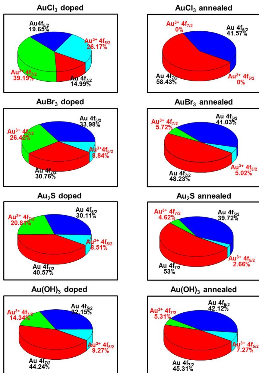
**Figure SI4.** The Au 4f peak separation was investigated. In the case of the Au complex doped graphene, the AuCl<sub>3</sub> had the largest ion peak, which was related to the degree of the decrease in the sheet resistance. But annealed AuCl<sub>3</sub> doped graphene sheet contained no gold ion peaks, indicating that they were completely degraded by thermal annealing.
