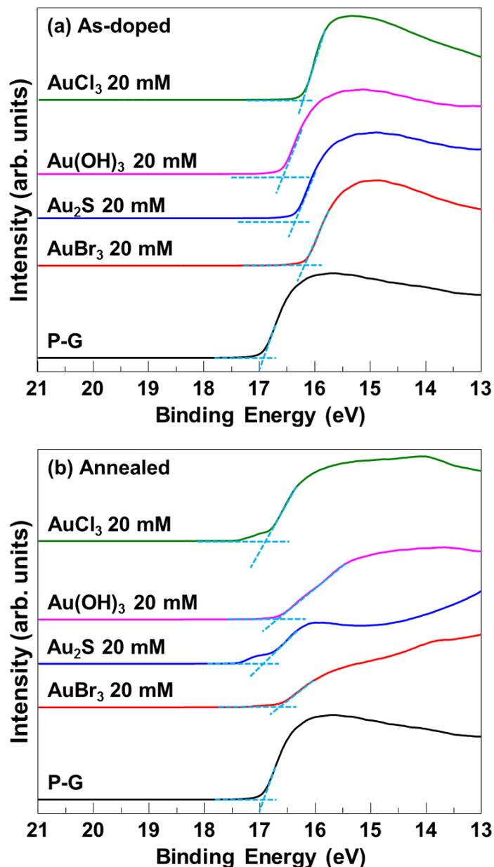
**Figure S15.** The UPS spectra shows the secondary electron threshold energy differences. The AuBr<sub>3</sub> doped graphene sheets had the lowest secondary electron threshold energy value, indicating that they have the highest work function value. But the annealed graphene sheets had a larger secondary electron threshold energy value than that of each doped graphene sheets. The AuCl<sub>3</sub> doped graphene had the largest variance among the Au complex doped graphene sheets.
