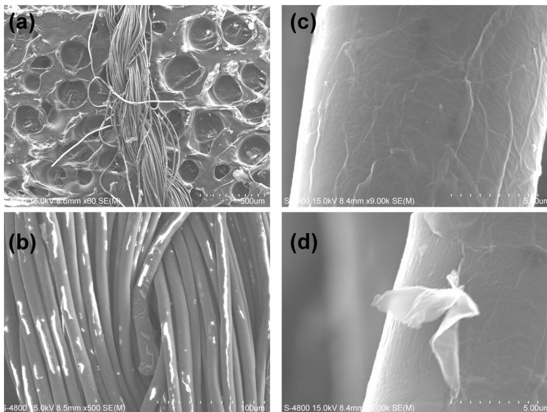
Fig. S6. SEM images of the cotton wire coated with GOLR. It can be seen that GOLR was tightly wrapped on surface of the wire. Those images were captured by scanning electron microscopy (SEM) (Hitachi S-4800, Hitachi, Ltd., Tokyo, Japan).
