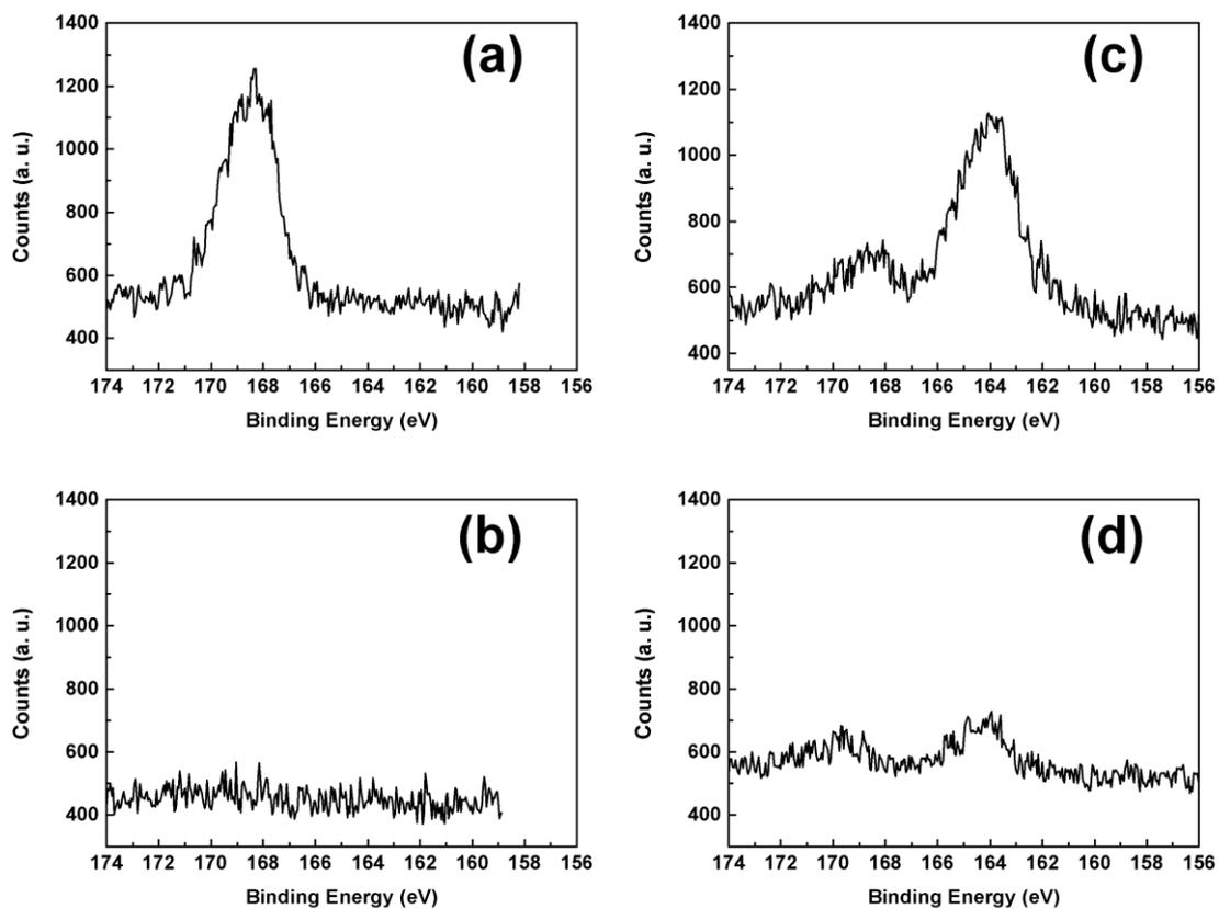
Fig. S3. XPS spectra of S2p of (a) GO, (b) GO300, (c) GOLR and (d) GOLR300.
