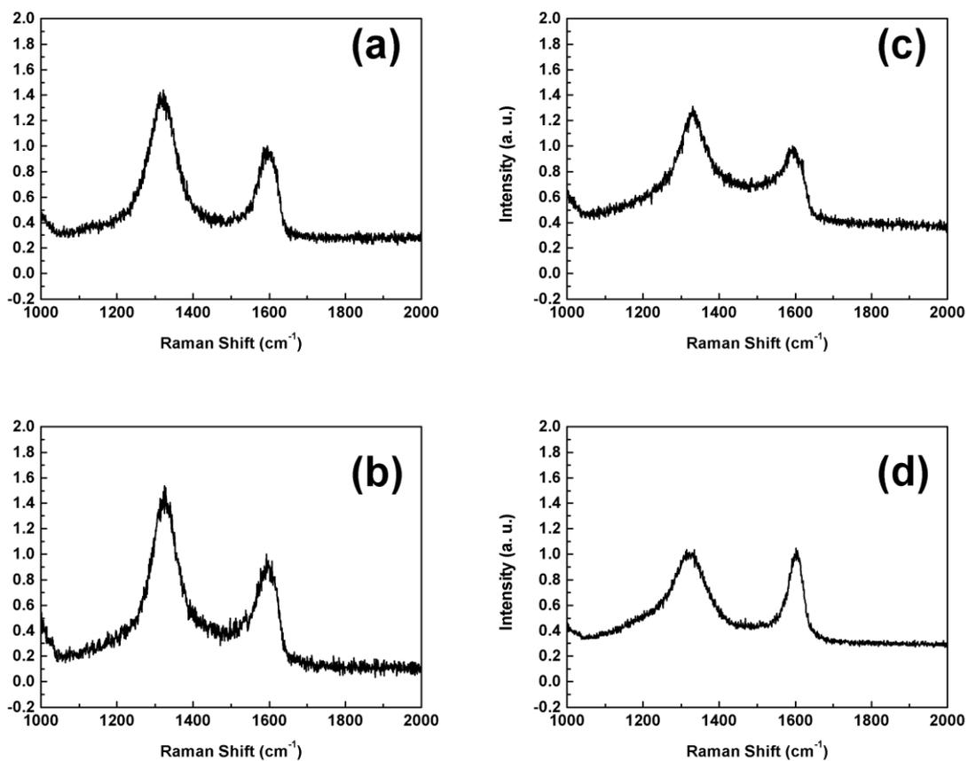
Fig. S4. Raman spectra of (a) HRGO, (b) GO300, (c) GOLR300 and (d) GO900, normalized at G bands.
