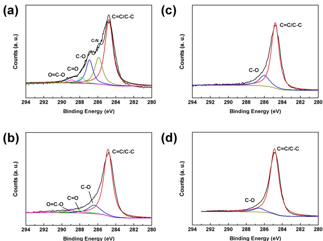
Fig. S1. Normalized XPS spectra of C1s peaks of (a) HRGO, (b) GO300, (c)
