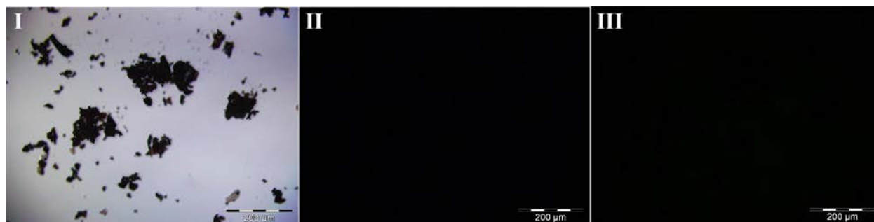
Figure S4. Shows the fluorescence microscopic images of powder as-prepared \text{Mn}_3\text{O}_4 NPs under irradiation of white light (I, bright field) and light of two different wavelengths of 365 (II) and 436 nm (III), respectively.
