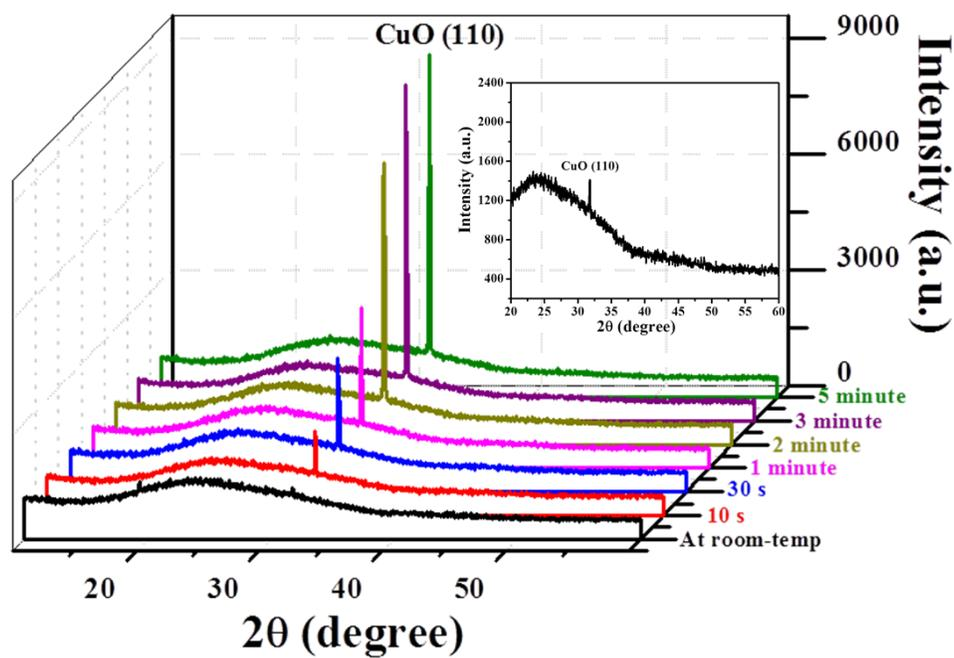
**Figure S6.** Typical X-ray diffraction patterns for the printed CuO nanofilms after microwave-assisted annealing (MAA) at different times. CuO nanofilms were printed using ink C. In inset showing magnified XRD pattern of CuO nanofilms at room-temperature
