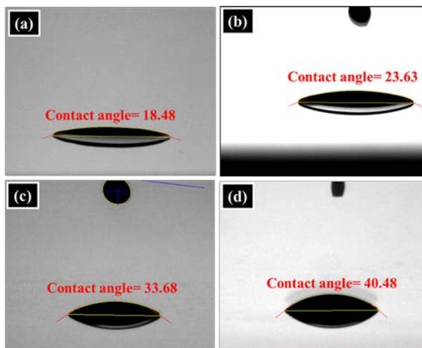
**Figure S4.** Contact angle of droplets using as-formulated CuO ink C on various substrates i.e. (a) Si/SiO<sub>2</sub>, (b) Bare glass, (c) PI and (d) ITO.
