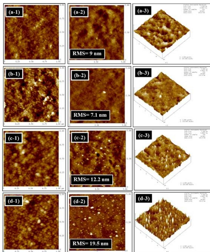
**Figure S5.** AFM images of CuO nano-films after conventional annealing at different temperatures: (a) 100 °C, (b) 150 °C, (c) 200 °C, and (d) 250 °C. CuO lines were printed using ink C.
