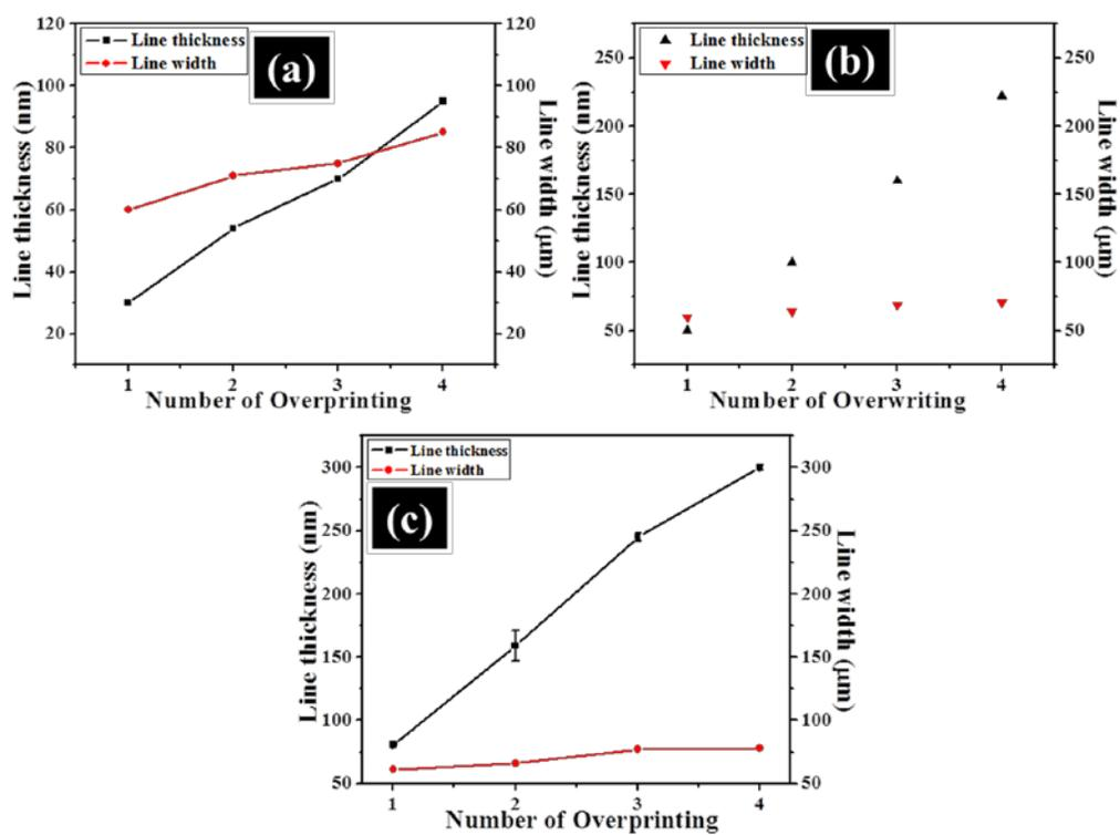
**Figure S3.** CuO line thickness and line width as a function of number of overprinting using (a) ink A, (b) ink B and (c) ink C.
