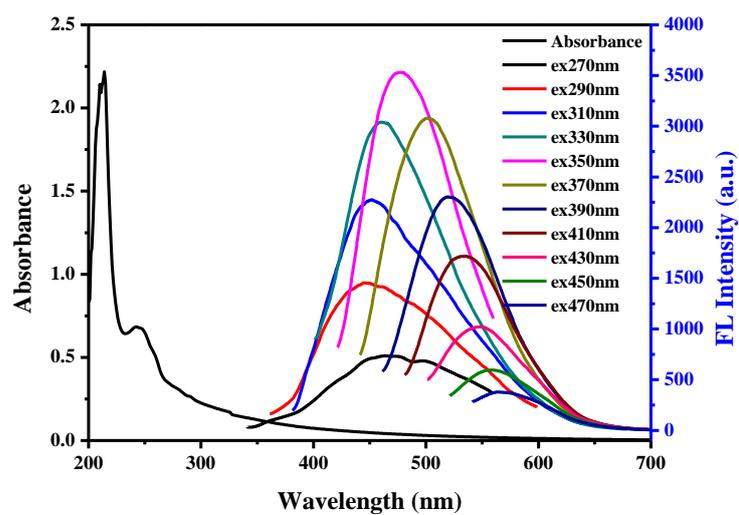
Fig. S4. Absorption spectrum the ethylenediamine-functionalized CNPs (CNP-en) and its fluorescence emission spectra at different excitation wavelengths when dispersed in ethanol.
