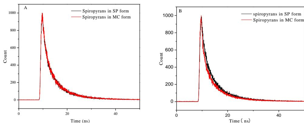
Fig. S6. The time-resolve fluorescence spectra of the physical mixture of CNPs-en and spiorpyrans (A) and CNPs-SP (B), when spiorpyrans are in SP or MC form. (The excitation is 405 nm, the emission is 510 nm)
