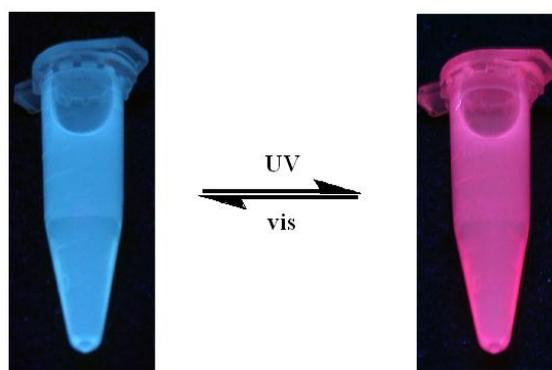
Fig. S5. The photographs of the spiropyrans-functionalized CNPs (CNP-SP) under 365 nm lamp dispersed in ethanol after irradiated with visible (left) and UV (365 nm) light (right) respectively.
