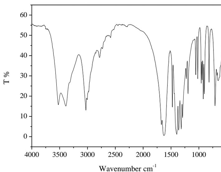
Fig.S1. The FTIR spectrum of EDTA.2Na
