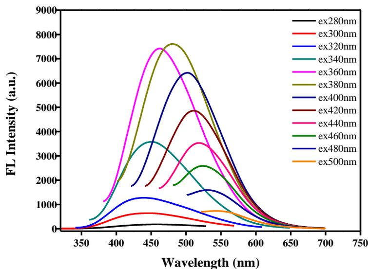
Fig. S3. The fluorescence emission spectra of the CNPs dispersed in water with different excitation wavelengths.
