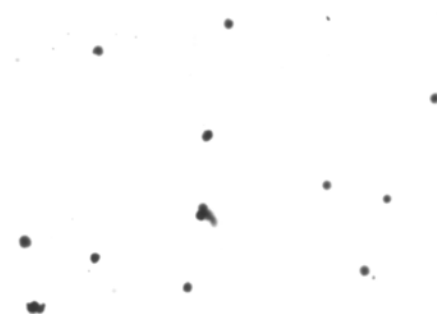
Fig. S6 An optical image of the \text{Fe}_3\text{O}_4@/\text{SiO}_2@/\text{Ag} microspheres
