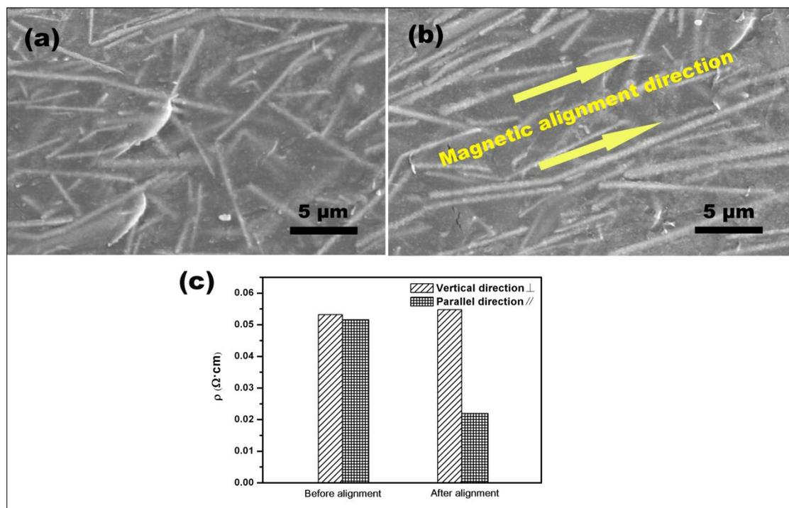
**Fig. S3** SEM images (a) before and (b) after magnetic field alignment and (c) electrical resistivity of the Fe<sub>3</sub>O<sub>4</sub>-coated Ag-NW/PVA composite film, in which MR=0.1:1 and Ag NW content = 2 wt% in the composite. The direction of the magnetic alignment is indicated by the arrows.
