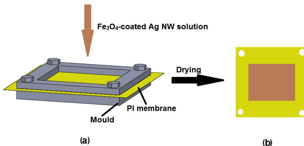
**Fig. S2** Schematic showing for preparation of Fe<sub>3</sub>O<sub>4</sub>-coated Ag NW films on the PI membrane.
