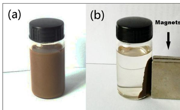
**Fig. S1** Digital photos of the ethanol solution containing  $\text{Fe}_3\text{O}_4$ -coated Ag NWs (MR=0.1:1): (a) before and (b) after placement of permanent magnets.
