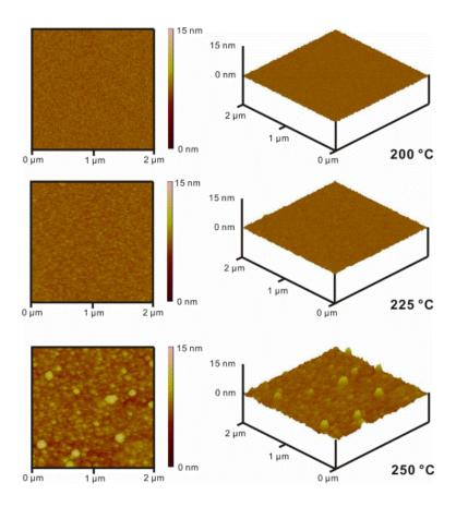
RMS roughness = 0.3 nm @ 200 °C, 0.4 nm @ 225 °C and 0.6 nm @ 250 °C
