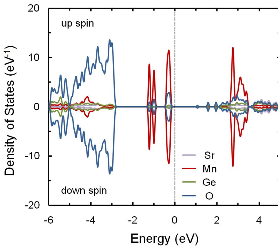
Figure S5. Calculated partial density of states for Sr, Mn, Ge, O in Sr<sub>2</sub>MnGe<sub>2</sub>O<sub>7</sub>. The Fermi level is set to zero.
