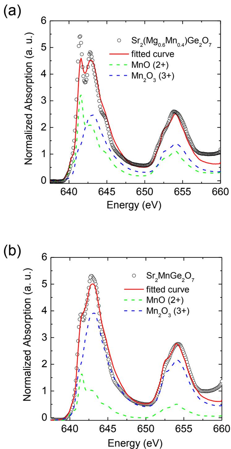
Figure S2. Fitted curves for Mn *L*-edge XANES spectra from (a)  $\text{Sr}_2(\text{Mg}_{0.6}\text{Mn}_{0.4})\text{Ge}_2\text{O}_7$  and (b)  $\text{Sr}_2\text{MnGe}_2\text{O}_7$  by the linear combination of *L*-edge spectra from MnO(2+) and  $\text{Mn}_2\text{O}_3$ (3+).
