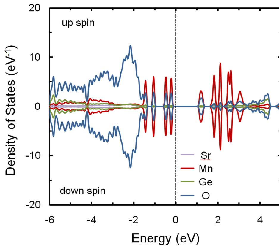
Figure S4. Calculated partial density of states for Sr, Mn, Ge, O in Sr<sub>2</sub>MnGe<sub>2</sub>O<sub>7.5</sub>. The Fermi level is set to zero.
