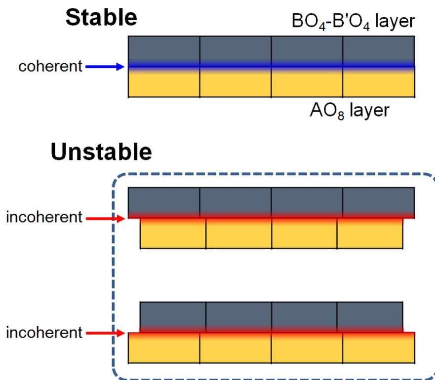
Figure S6. Schematic expression for the stability of the melilite structure determined by the coherency between  $BO_4-B'O_4$  and  $AO_8$  layers in  $A_2BB'_2O_7$ .
