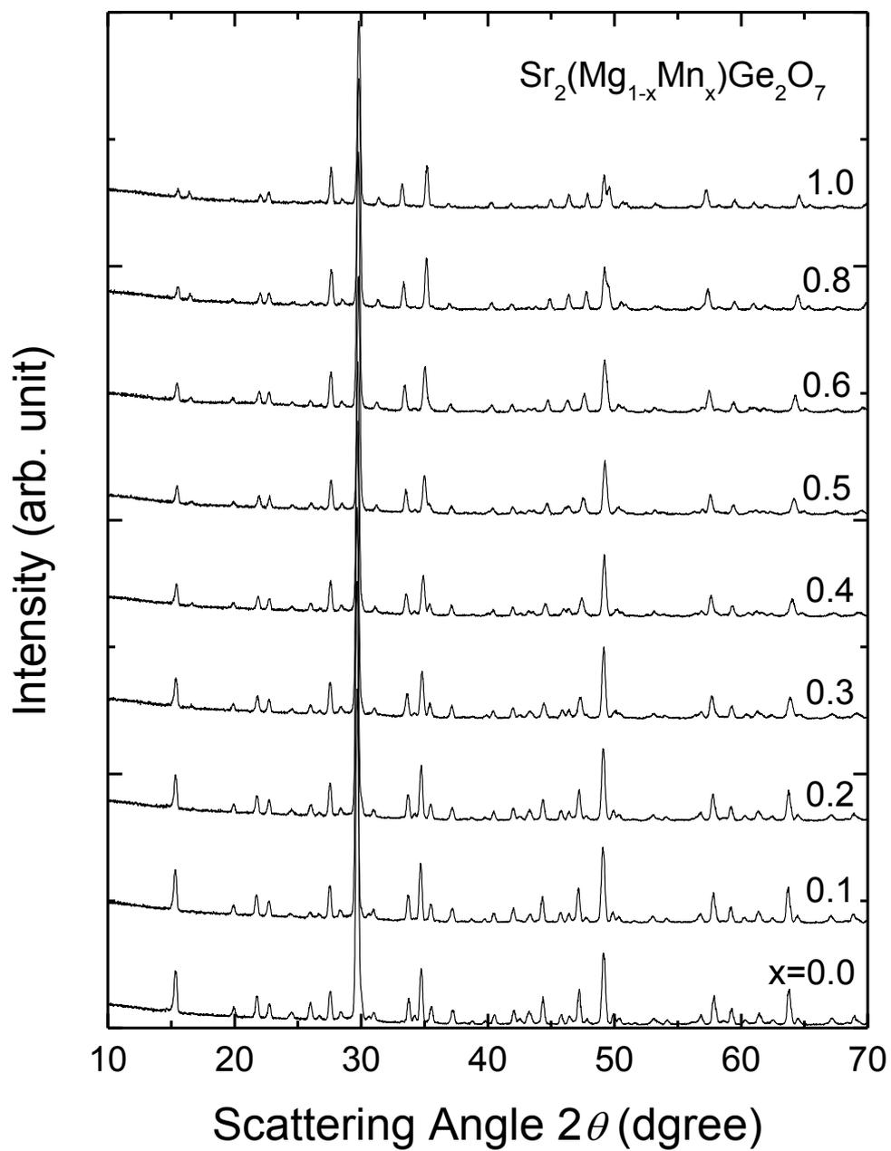
Figure S1. X-ray diffraction patterns of  $\text{Sr}_2(\text{Mg}_{1-x}\text{Mn}_x)\text{Ge}_2\text{O}_7$  ( $x = 0.0, 0.1, 0.2, 0.3, 0.4, 0.5, 0.6, 0.8$  and 1.0) powders.
