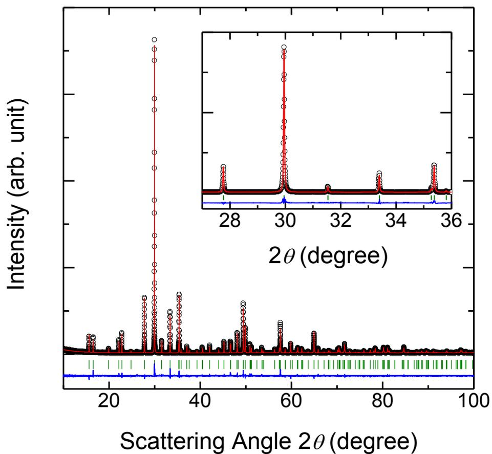
Figure S3. Rietveld refinement of the synchrotron powder XRD profile of  $\text{Sr}_2\text{MnGe}_2\text{O}_{7.5}$  including a O4 oxygen interstitial atom. Measured data, fitted results, expected reflection positions, and the difference between measured and fitted results are expressed as black open circles, red solid lines, green vertical lines, and blue solid lines, respectively.
