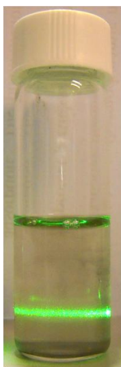
Figure S4. Tyndall effect confirming the colloidal nature of the exfoliated graphene dispersions after standing for one month.
