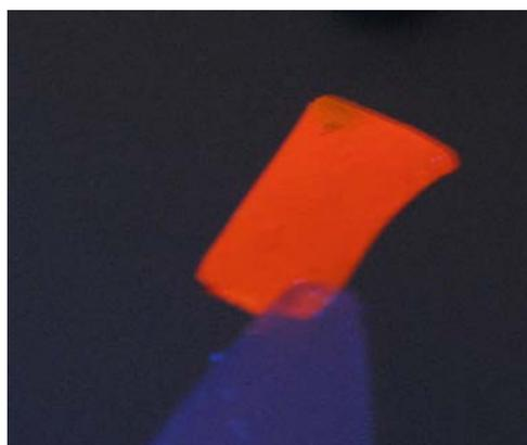
**Figure S1.** Photograph of stain etching-derived porous silicon under 365 nm excitation from a hand-held lamp.
