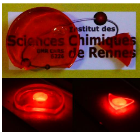
Figure4s: Picture of pieces of PM20 (left) and PM50 (right) under daylight (top) and UV irradiation at 350-380 nm (bottom). The thickness of both samples is 1.2mm and 0.8 mm for PM20 and PM50 respectively.
