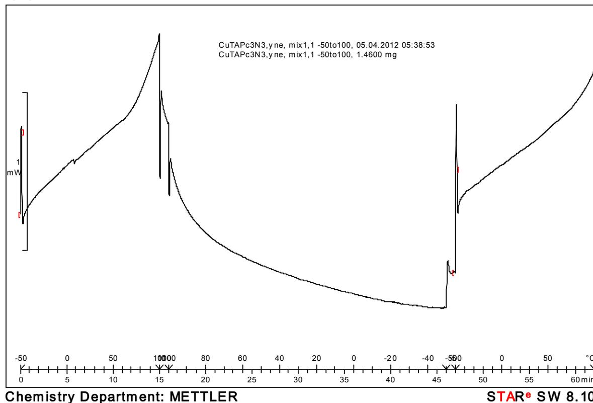
**Figure S29:** Low temperature DSC (10 °C/min, N<sub>2</sub>) of a freshly prepared 1:1 (mol/mol) mixture of **6aCu** and **7aCu**. No phase transitions are observed but the baseline rises exothermally, especially at temperatures above 80 °C, which is attributed to the exothermic click reaction.
