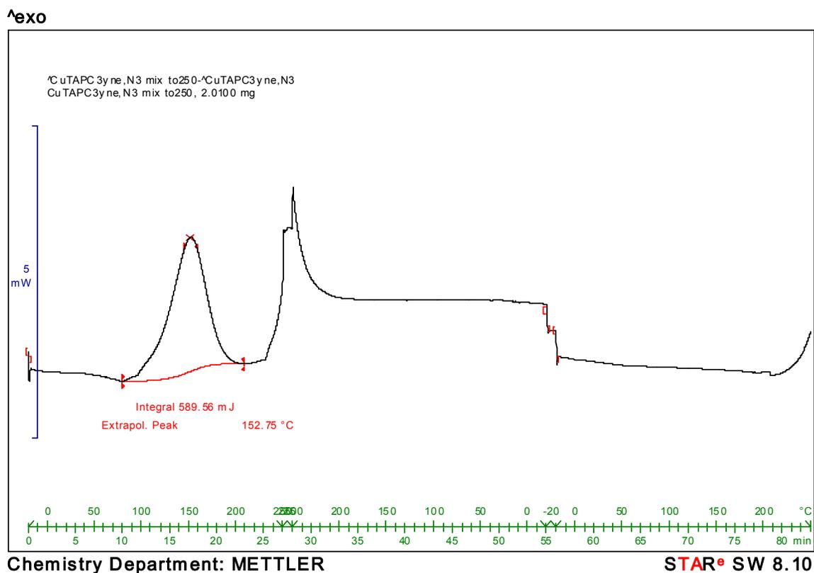
**Figure S30:** High temperature DSC (10 °C/min, N<sub>2</sub>, baseline subtracted) of a freshly prepared 1:1 (mol/mol) mixture of **6aCu** and **7aCu**. The large exothermic peak (293 J/g) is attributed to the exothermic click reaction. The rise of the baseline above 200 °C is likely caused by thermal decomposition.
