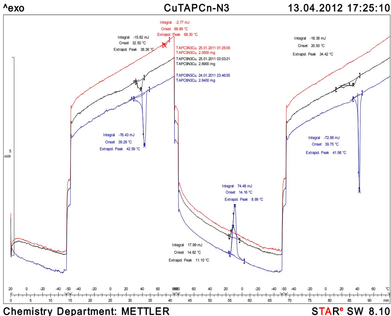
**Figure S14:** DSC graphs and analysis of **6aCu** (red), **6bCu** (blew), and **6cCu** (black) at 10 °C/min under N<sub>2</sub>. Compounds **6aCu** and **6bCu** display Col<sub>h</sub> mesophases but the clearing temperature of **6aCu** is larger than its onset of decomposition at 117 °C and the clearing transition of **6bCu** is not observed by DSC.
