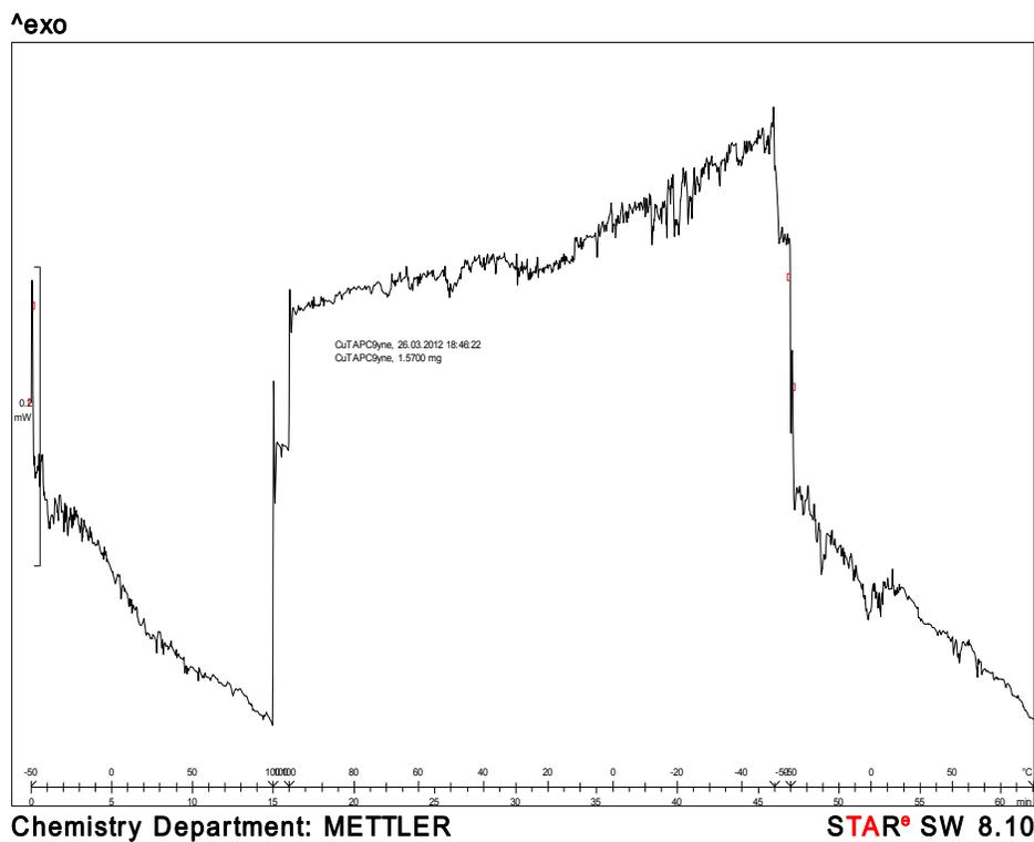
**Figure S20:** DSC graph of **7cCu** at 10 °C/min (heating) and 5 °C/min (cooling) under N<sub>2</sub>. No transitions are observed.
