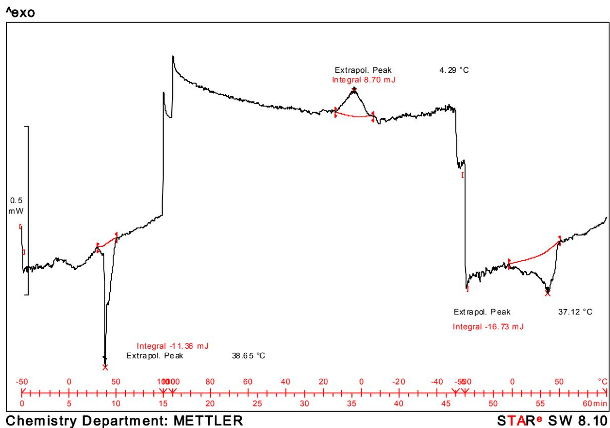
Figure S17: DSC graph and analysis of **7c** at 10 °C/min (heating) and 5 °C/min (cooling) under N<sub>2</sub>.
