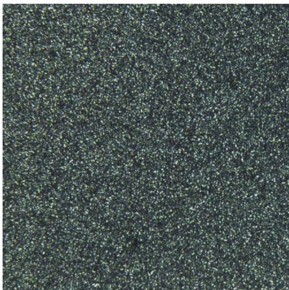
**Figure S28:** POM micrograph of **7aCu** between glass slides at 100 °C (200x). The domain size is very small and the resulting texture is not characteristic for a specific type of mesophase.
