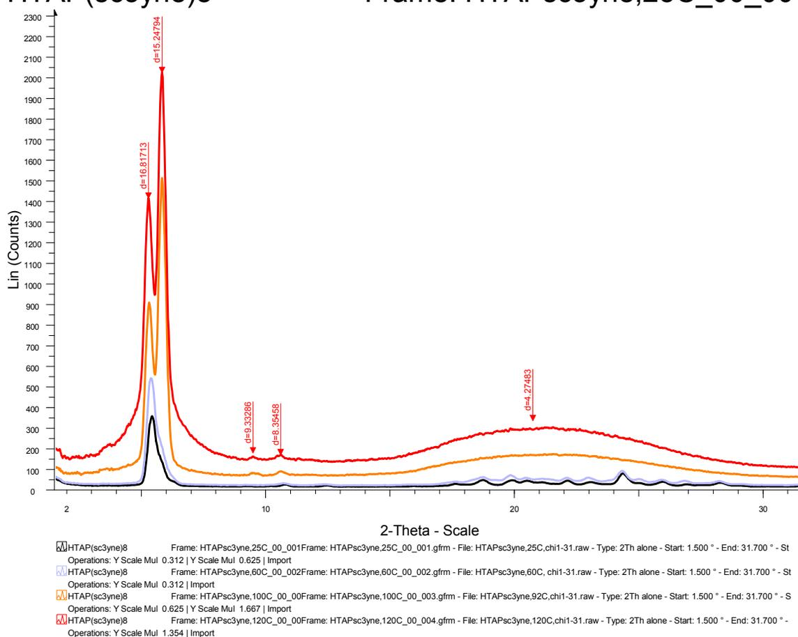
**Figure S23:** pXRD graphs of the crystalline phase of **7a** at 25 °C (black) and 60 °C (purple) and of its Col<sub>r</sub> mesophase at 100 °C (orange) and 120 °C (red).
