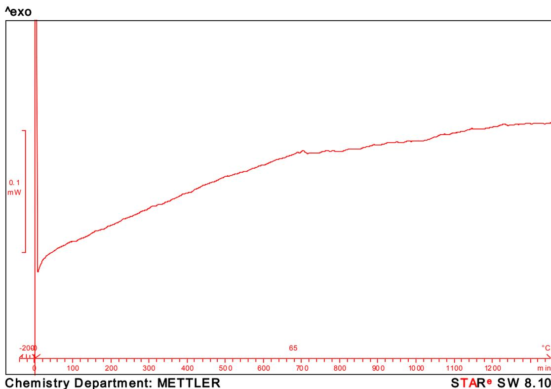
**Figure S31:** Isothermal DSC run (heated to 65 °C at 10 °C/min and then isothermal for 2 days, N<sub>2</sub>) of a freshly prepared 1:1 (mol/mol) mixture of **6aCu** and **7aCu**. The positive slope of the curve is attributed to the exothermic click reaction. Progress of the reaction appears to be faster in the first 700 minutes (steeper slope) and then gradually slowing down until it is almost zero after about 1300 minutes (22 hours).
