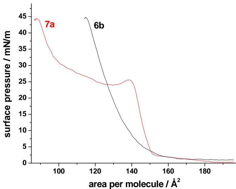
Fig. S32 Surface pressure area isotherms of TAPs **6b** and **7a** on pure water at pH = 6.5 and 25 °C.
