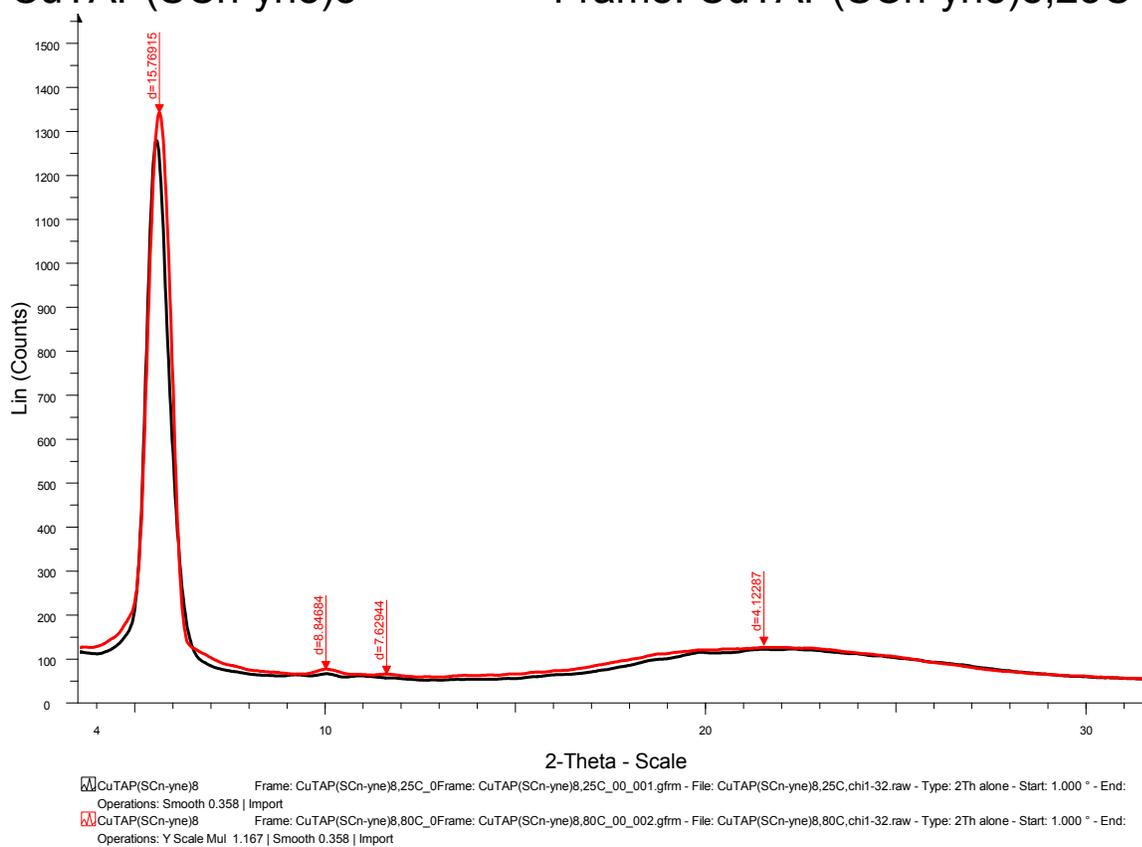
**Figure S24:** pXRD graphs of the crystalline phase of **7aCu** at 25 °C (black) and of its Col<sub>h</sub> mesophase at 80 °C (red).
