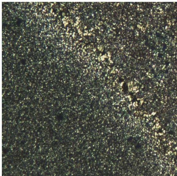
**Figure S25:** POM micrograph of **6aCu** between glass slides at 100  $^{\circ}\text{C}$  (200x). The domain size is small but some areas of fan-shaped textures are observed that are characteristic for columnar mesophases.
