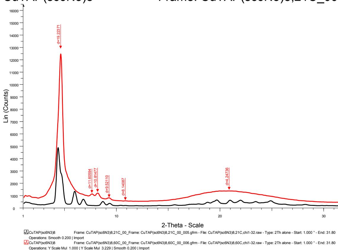
**Figure S22:** pXRD graphs of **6bCu** at 21 °C (black line, crystalline phase) and 60 °C (red line, Col mesophase). The reflections as assigned do not agree with a Col<sub>h</sub> mesophase and a closer look at the shape of the small angle reflection at 19.22 Å reveals two reflections as it has a shoulder towards smaller angles. The peak positions of the two reflections are estimated to 20.415 Å and 18.981 Å.
