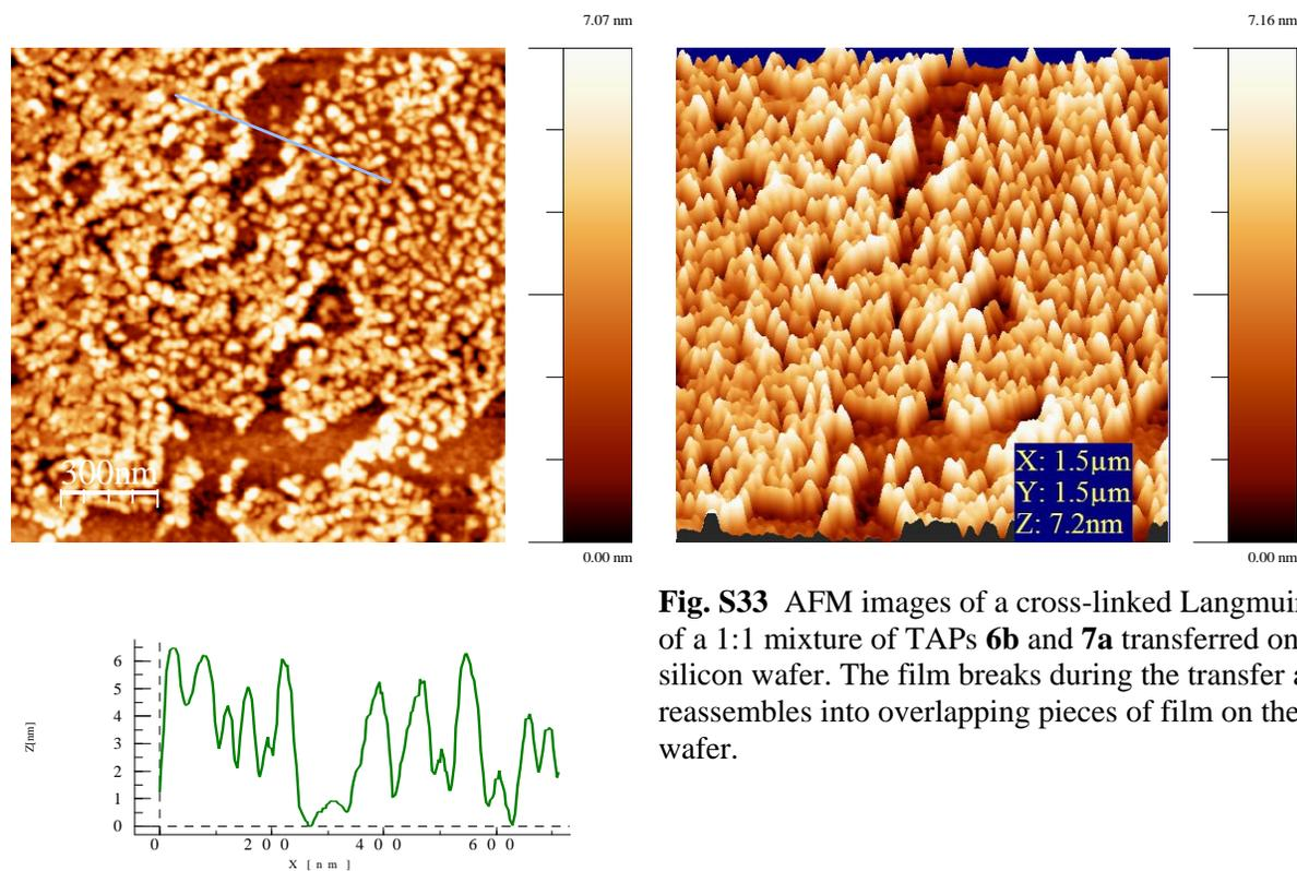
Fig. S33 AFM images of a cross-linked Langmuir film of a 1:1 mixture of TAPs **6b** and **7a** transferred onto silicon wafer. The film breaks during the transfer and reassembles into overlapping pieces of film on the wafer.
