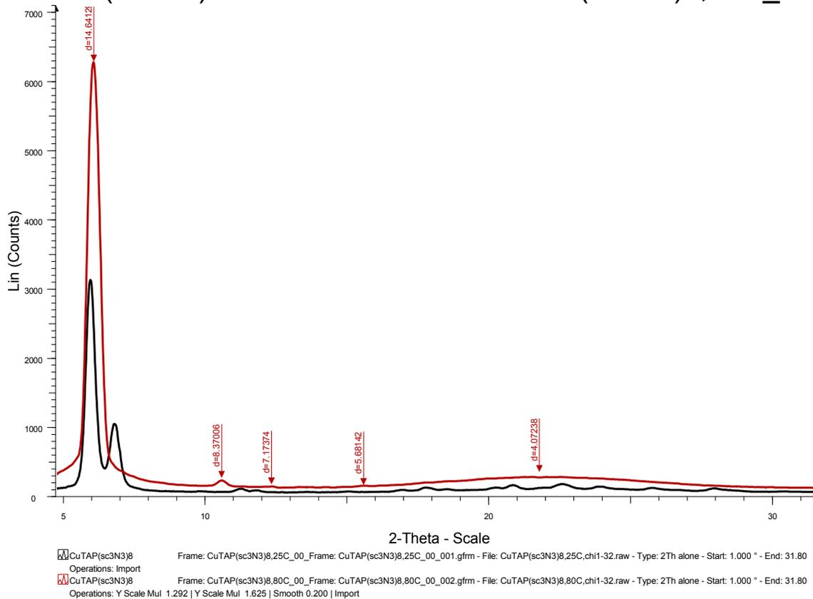
**Figure S21:** pXRD graphs of **6aCu** at 25 °C (black line, crystalline phase) and 80 °C (red line, Col<sub>h</sub> mesophase).
