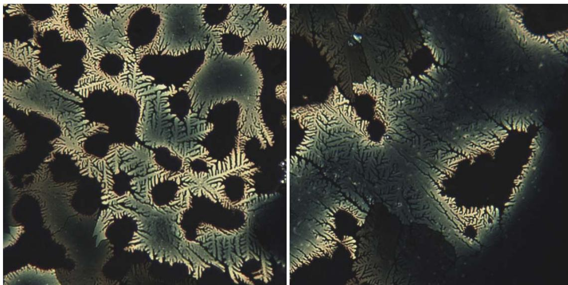
**Figure S26:** POM micrographs of **6bCu** as a thin film on glass at 41  $^{\circ}\text{C}$  (left) and 45  $^{\circ}\text{C}$  (right) on cooling from the isotropic liquid (200x). The dendritic growth textures are typical for  $\text{Col}_h$  and  $\text{Col}_r$  mesophases. Dark areas are free of compound due to local dewetting of the thin film (about 500 nm thick).
