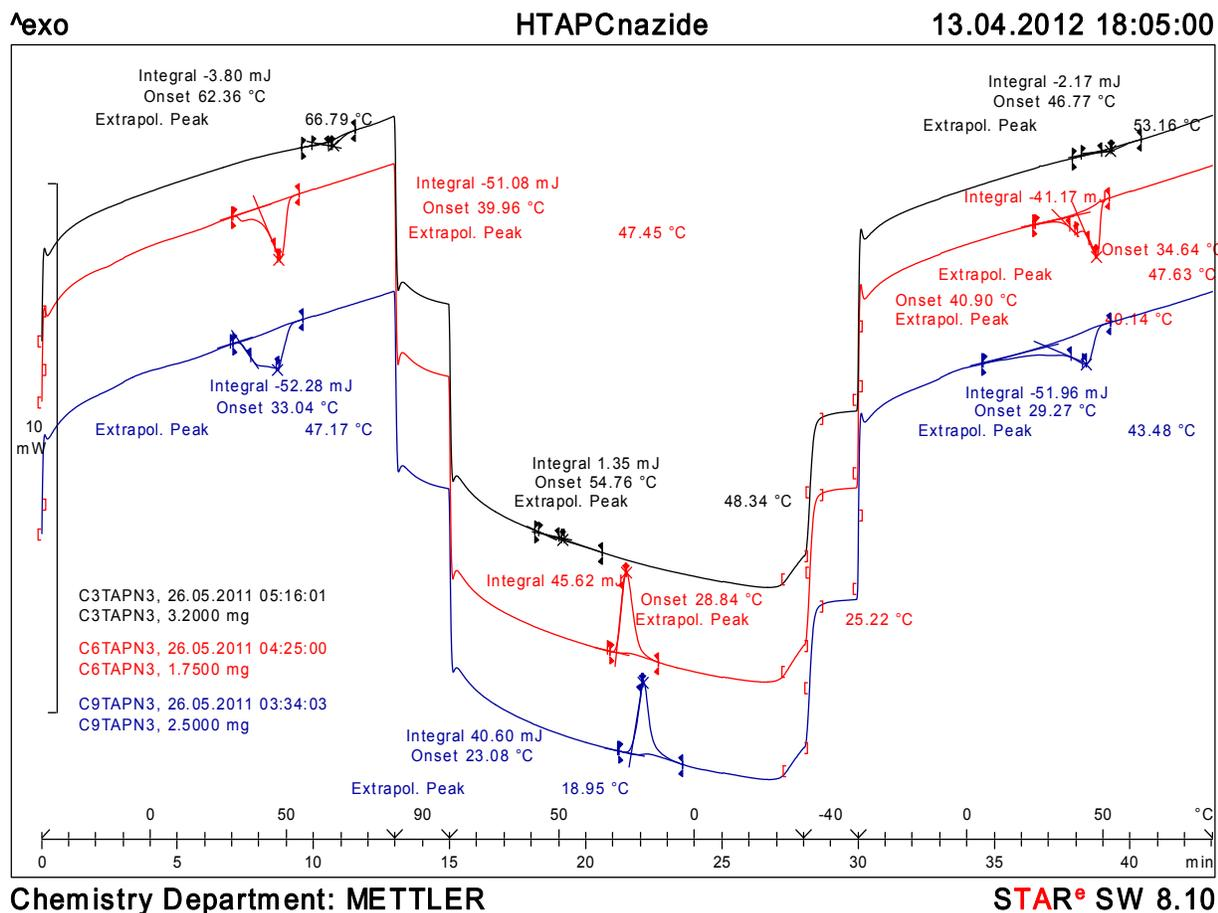
**Figure S13:** DSC graphs and analysis of **6a** (black), **6b** (red), and **6c** (blew) at 10 °C/min under N<sub>2</sub>. No mesophases were observed.
