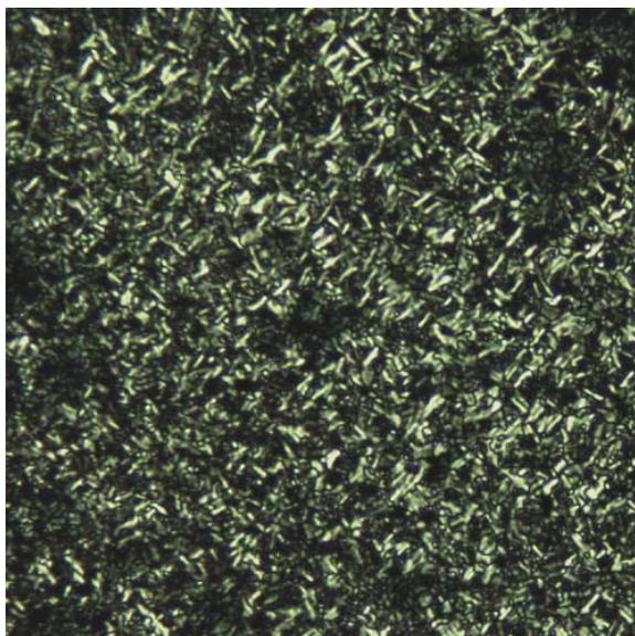
**Figure S27:** POM micrograph of **7a** as a thin film on glass at 120 °C on cooling from the isotropic liquid (200x). The observed fan-shaped texture is characteristic for columnar mesophases.
