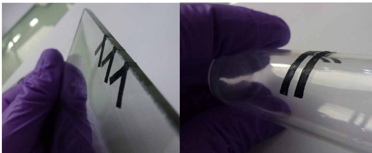
Figure S2. Pictures of PEDOT:PSS thick films transferred on thick glass and a curved plastic surface.
