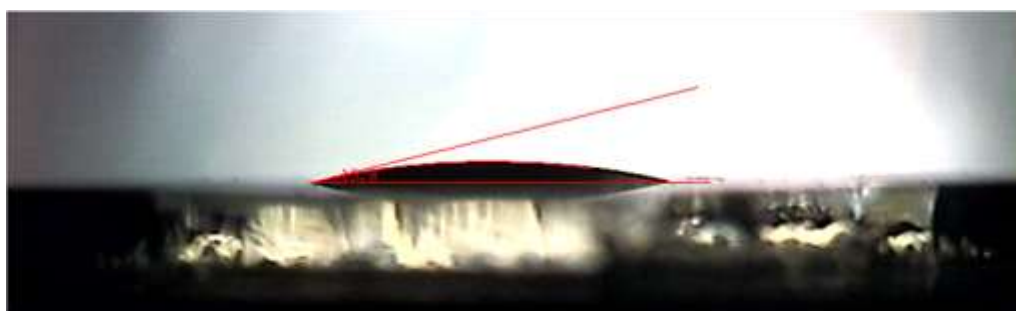
Figure S7. Contact angle of DCAE7T-F7 solution in \text{CHCl}_3 dropped on the ITO surface.
