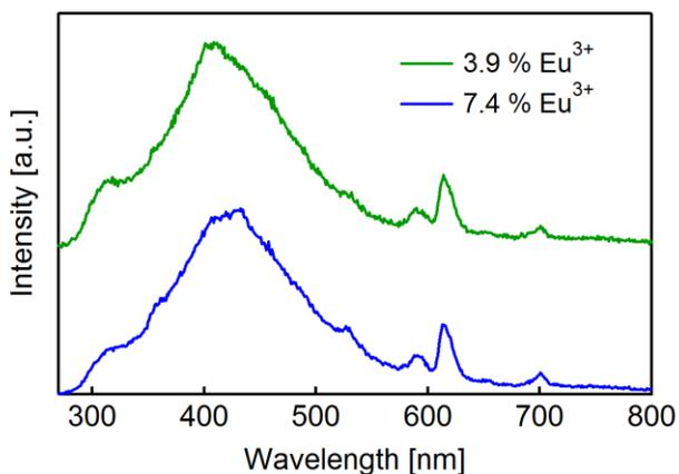
**Fig. S2** Steady-state PL spectra of highly  $\text{Eu}^{3+}$ -doped (3.9 and 7.4 % doping concentrations)  $\text{Ga}_2\text{O}_3$  NCs.  $\text{Eu}^{3+}$  intra-4f transitions are readily observed even in steady-state spectra.
