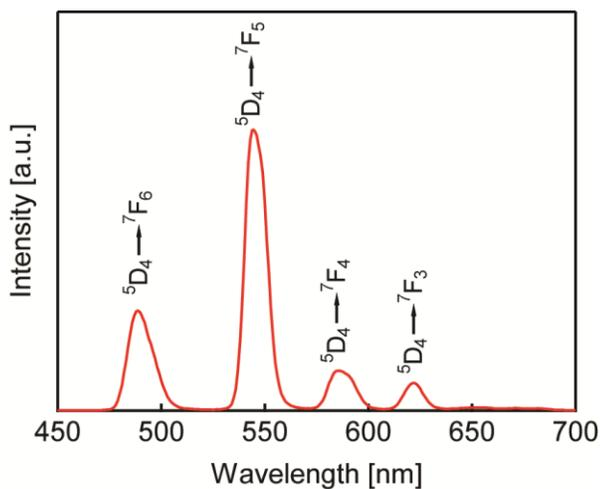
**Fig. S4** Time-gated PL spectrum of 10 %  $\text{Tb}^{3+}$ -doped  $\text{Ga}_2\text{O}_3$  NCs, showing the assignment of the observed f-f transitions.
