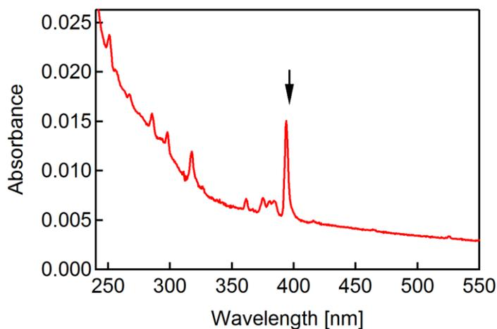
**Fig. S3** Typical electronic absorption spectrum of  $\text{Eu}^{3+}$  in an aqueous solution. The arrow indicates  ${}^7\text{F}_0 \rightarrow {}^5\text{L}_6$  transition used for direct excitation of  $\text{Eu}^{3+}$ .
