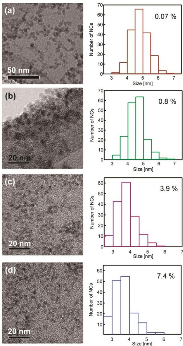
**Fig. S1** TEM images (left) and size distribution histograms (right) of  $\text{Eu}^{3+}$ -doped  $\text{Ga}_2\text{O}_3$  NCs with an average  $\text{Eu}^{3+}$  doping concentration of: (a) 0.07%, (b) 0.8%, (c) 3.9%, and (d) 7.4%.
