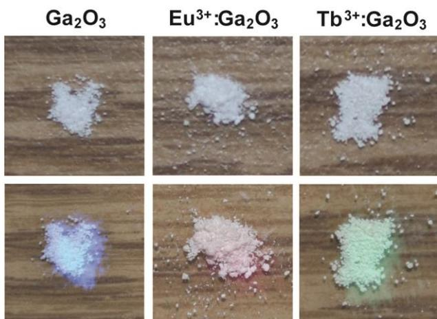
**Fig. S5** Photographs of  $\gamma$ - $\text{Ga}_2\text{O}_3$  (left), 7.4 %  $\text{Eu}^{3+}$ -doped  $\text{Ga}_2\text{O}_3$  (middle), and 10 %  $\text{Tb}^{3+}$ -doped  $\text{Ga}_2\text{O}_3$  NC powders (right). Top and bottom panels compare the day-light photographs of isolated samples (top), and the same samples illuminated with 250 nm UV light (bottom). The luminescence can be clearly observed even in day light.
