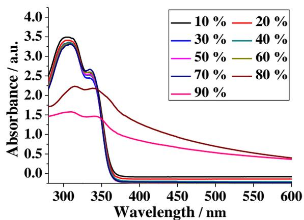
Fig. S9. UV-visible absorption spectra of WuFDA in mixed solvents of THF/H<sub>2</sub>O.
