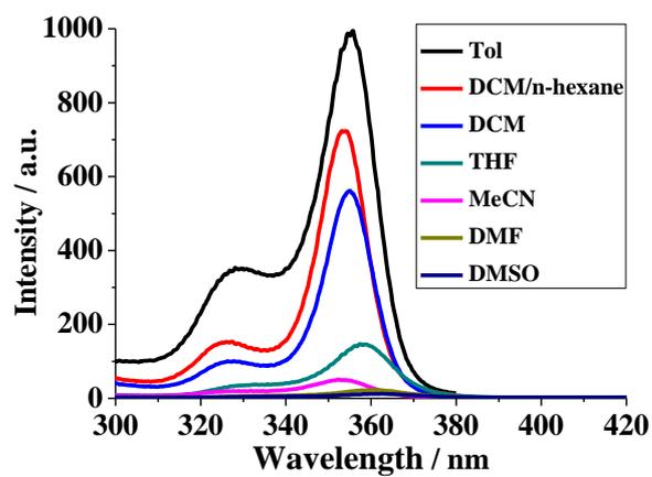
Fig. S8. Fluorescence excitation spectra of WuFDA in different solvents.
