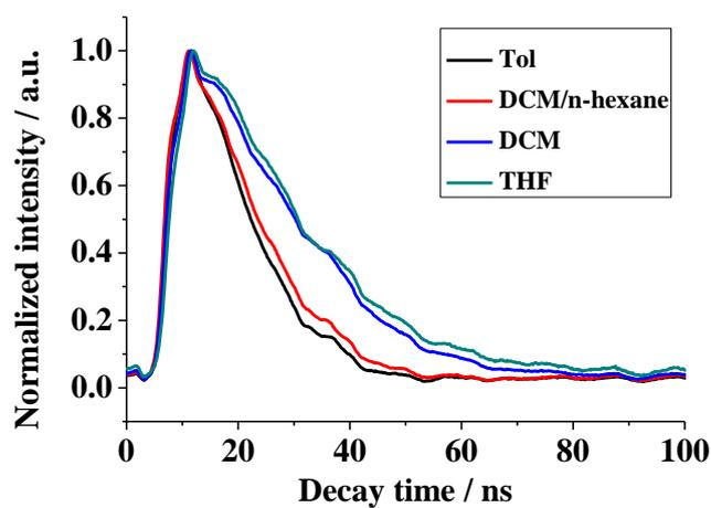
Fig. S4. Fluorescence decay curves of WuFDA in different solvents.
