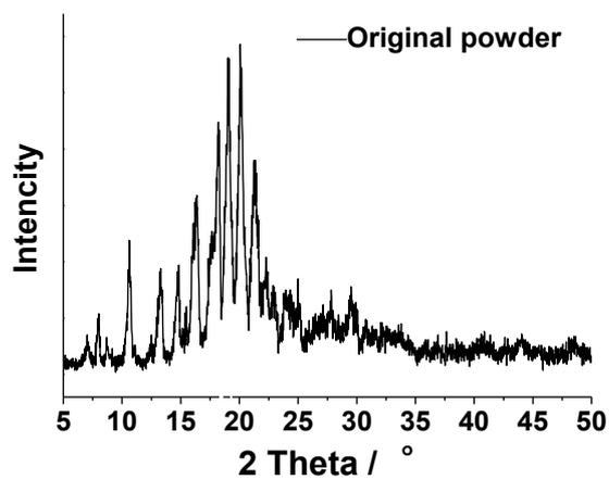
Fig. S6. WAXD pattern of the original powder of WuFDA.
