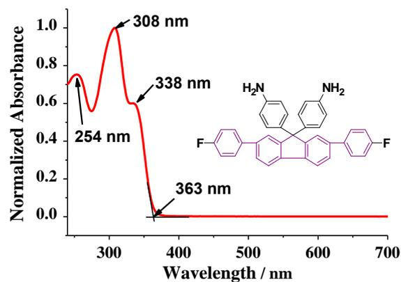
Fig. S3. UV-visible absorption spectrum of WuFDA in  $1 \times 10^{-5}$  mol/L THF solution.
